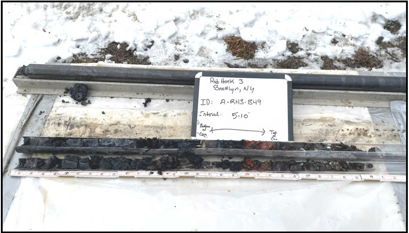
Photo 33: A-RH3-B49 – 5 to 10 feet with viscous creosote-like material at 8 to 10 feet
