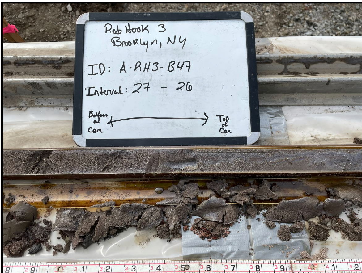
Photo 22: A-RH3-B47 – sheen and stained liner at 26 to 27 feet
