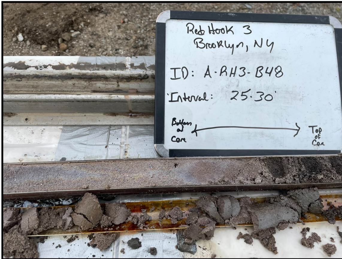
Photo 31: A-RH3-B48 – sheen and staining in liner at 26 to 27 feet
