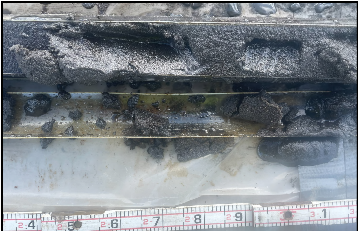
Photo 62: A-RH3-B52 – sheen and staining at 17 feet
