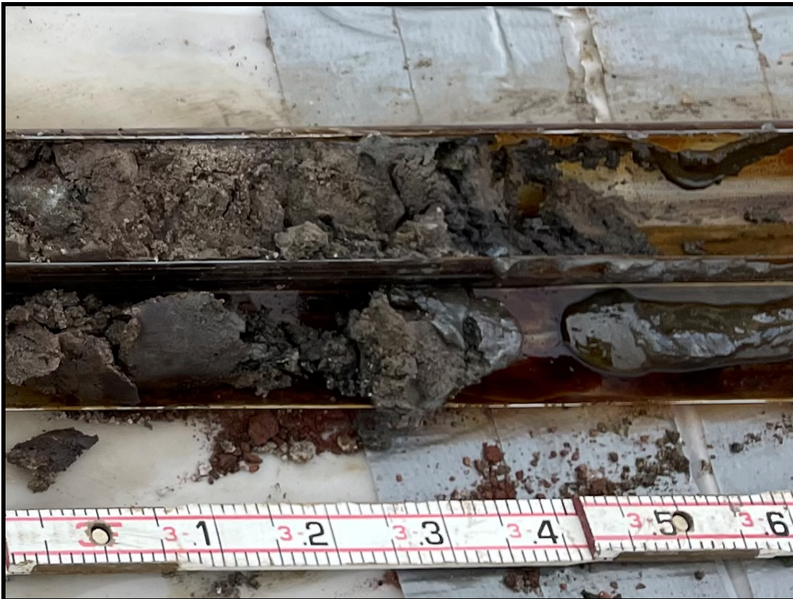
Photo 18: A-RH3-B47 – DNAPL saturated at 15 to 16 feet
