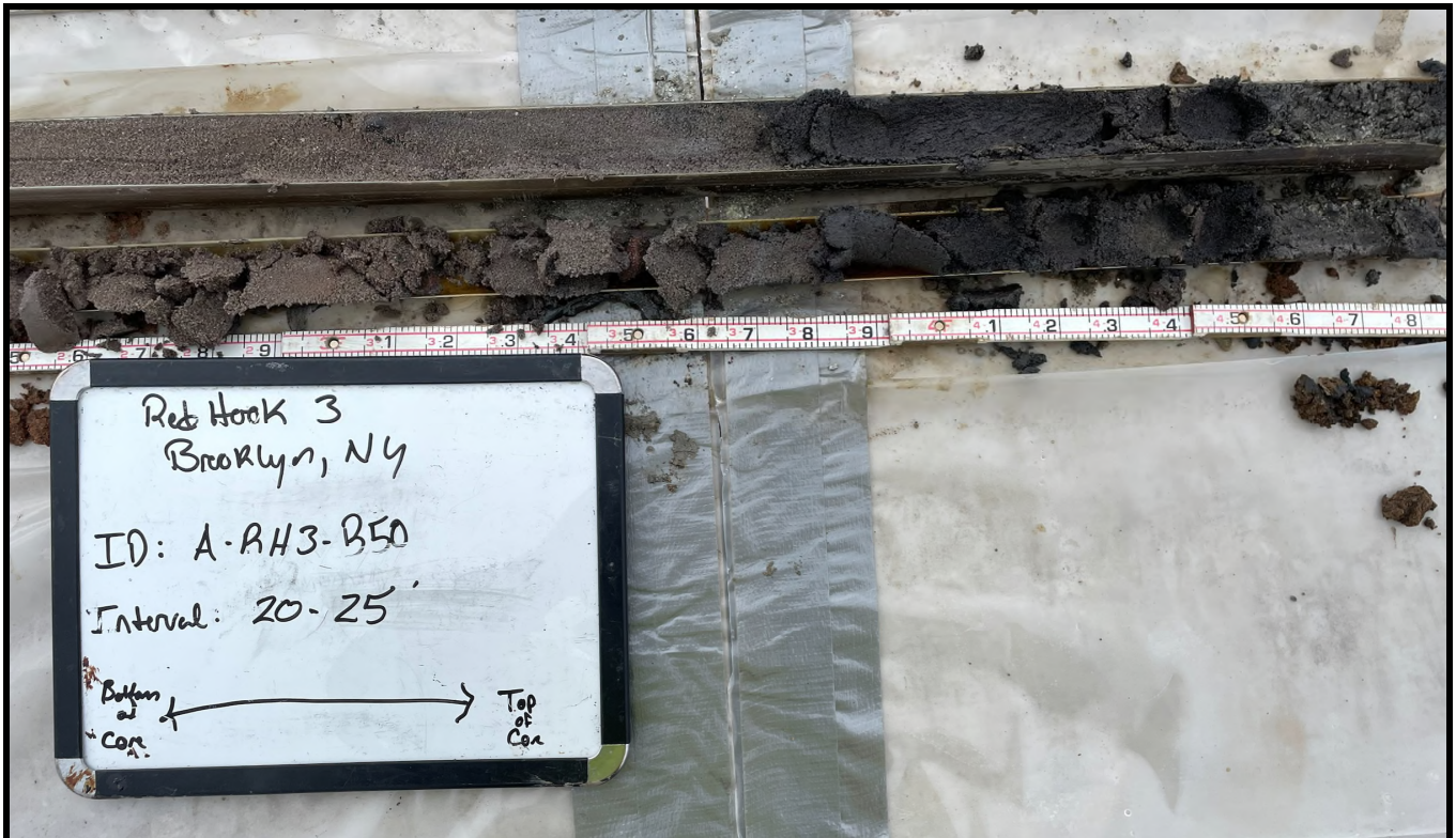
Photo 47: A-RH3-B50 – staining at 21.5 to 22 feet
