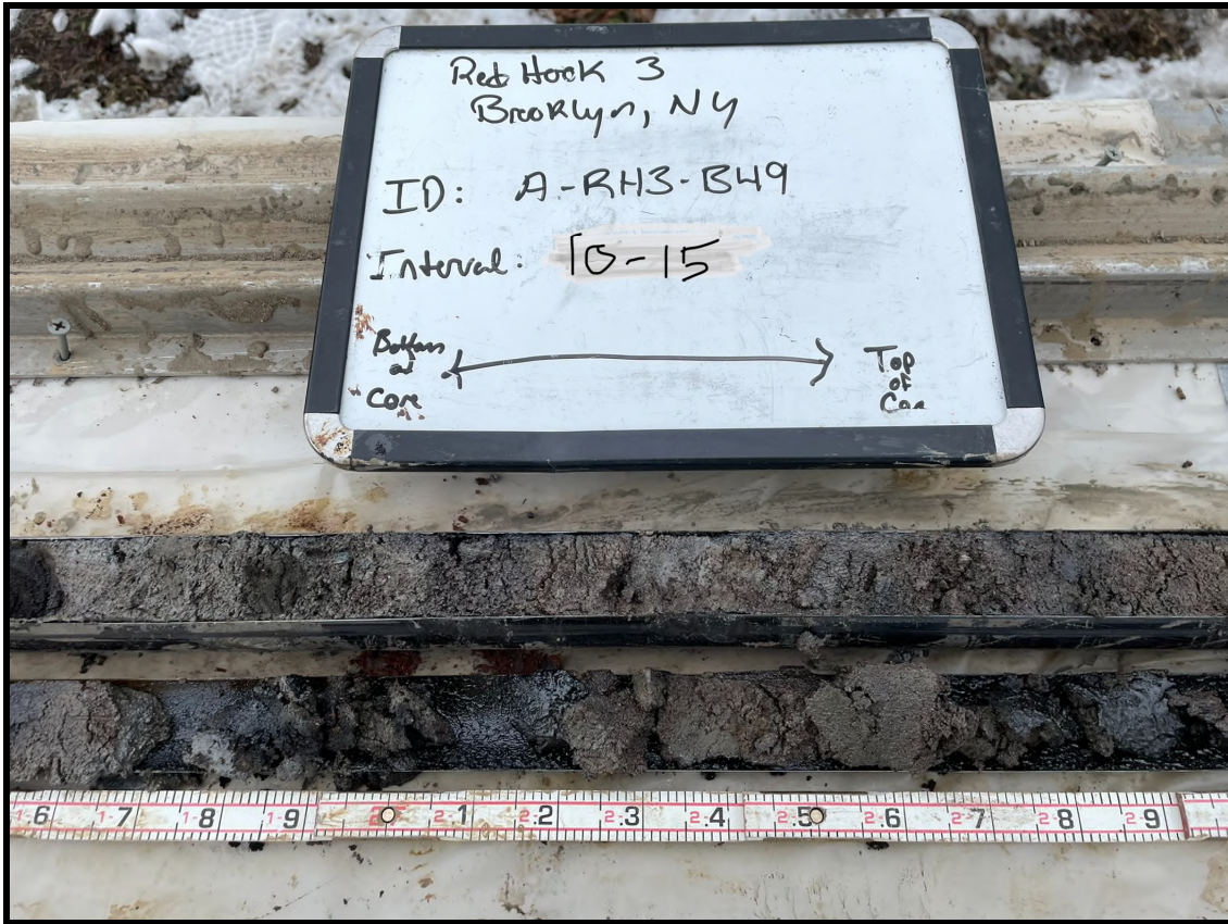
Photo 35: A-RH3-B49 – staining at 12 to 13 feet
