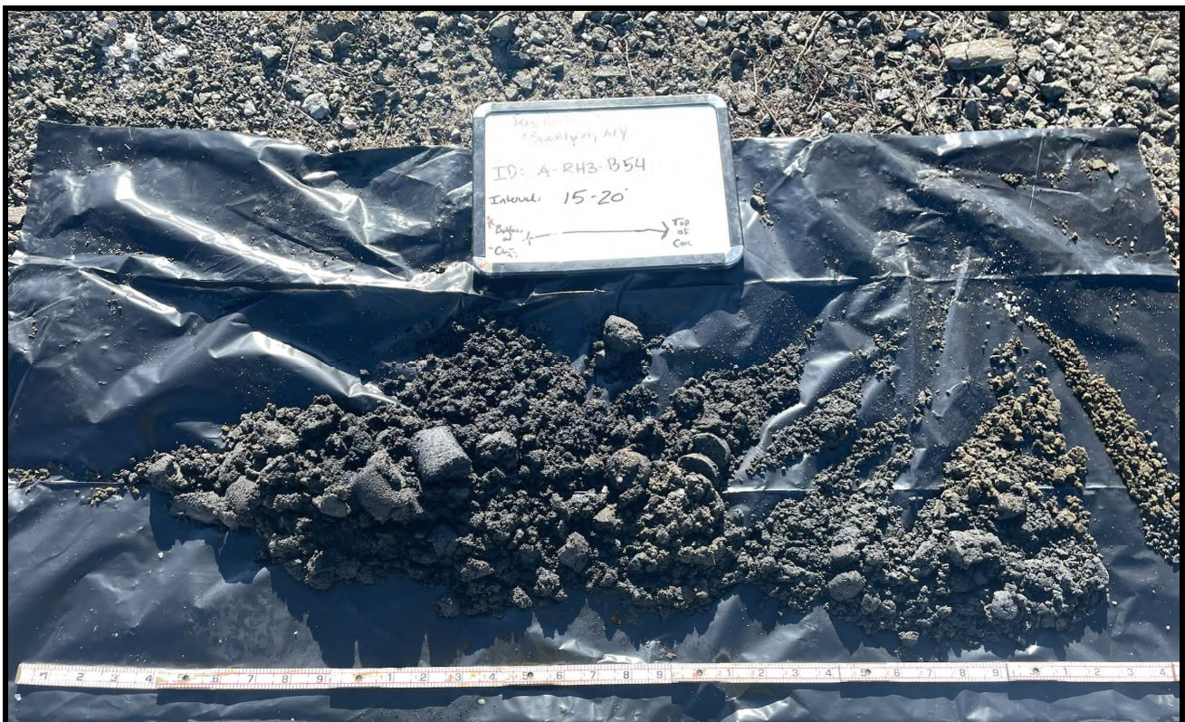
Photo 78: A-RH3-B54 – 15 to 20 feet (liner was stuck in core barrel – soil emptied onto sheet with hammer)
