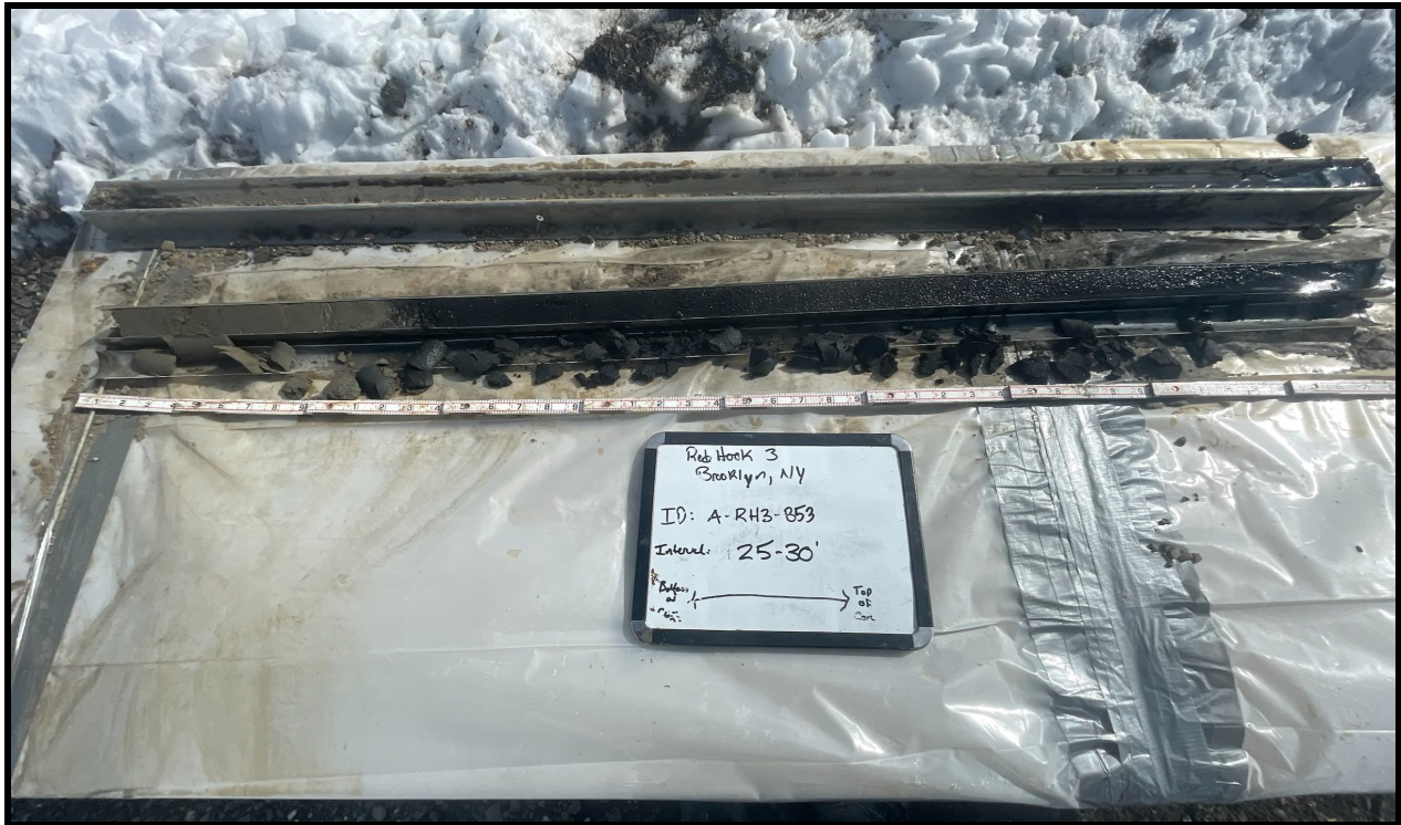
Photo 73: A-RH3-B53 – 25 to 30 feet with staining to 28.7 feet
