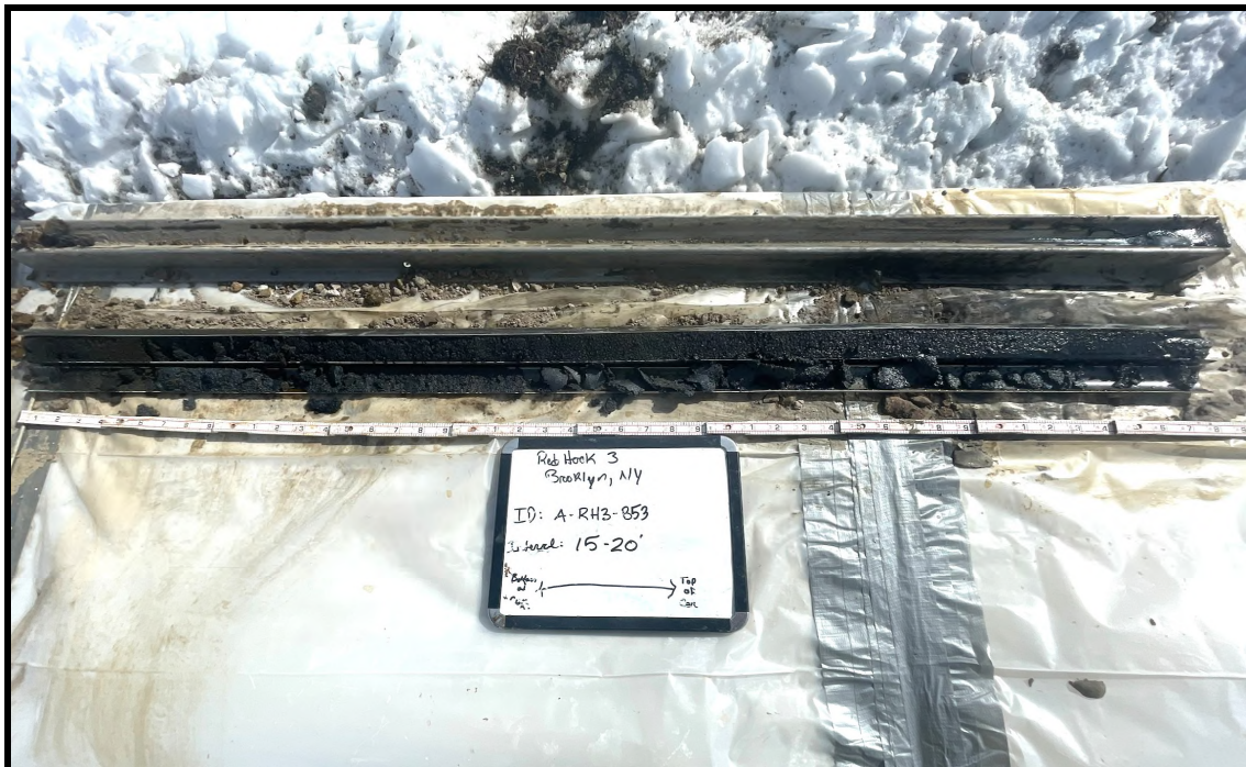
Photo 70: A-RH3-B53 – 15 to 20 feet showing staining
