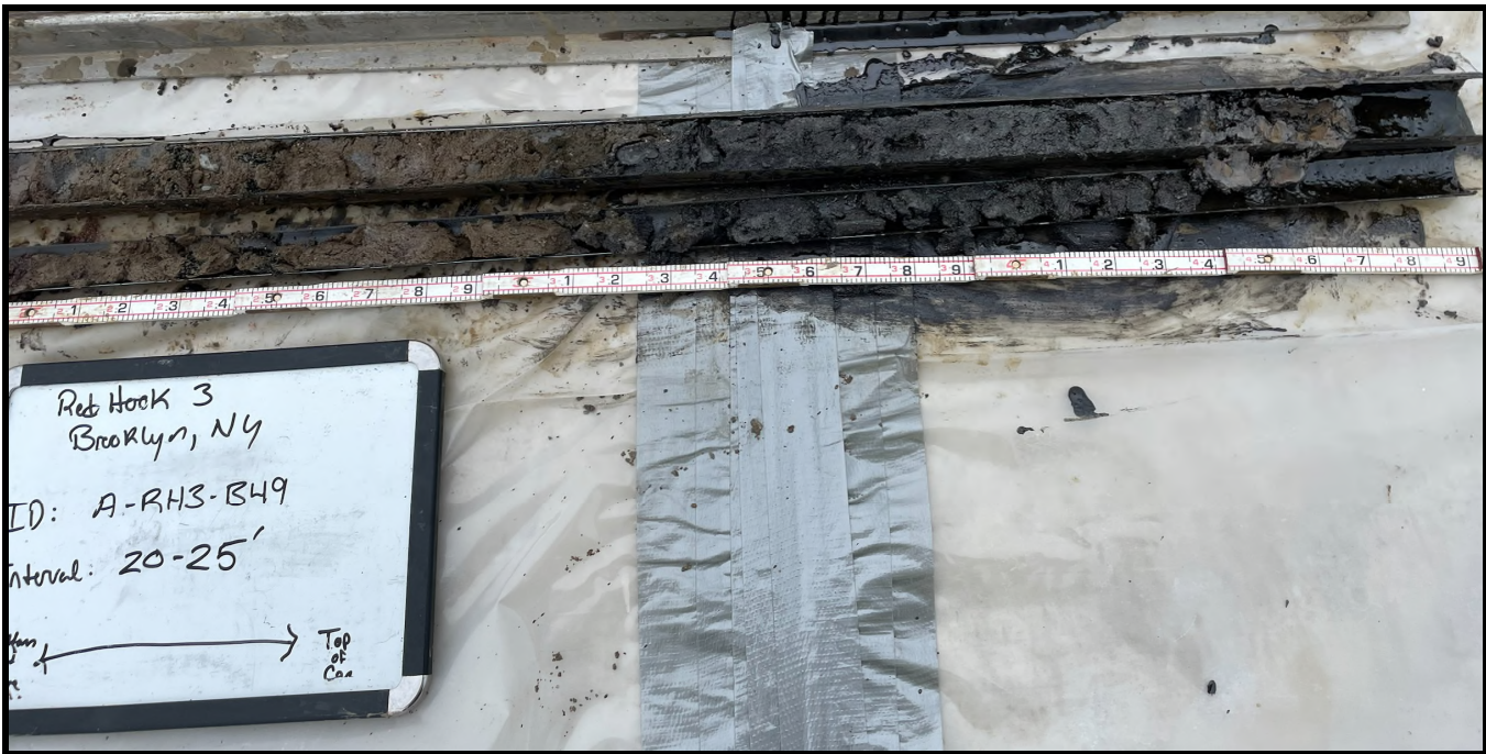
Photo 38: A-RH3-B49 – heavy staining at 20 to 21.5 feet
