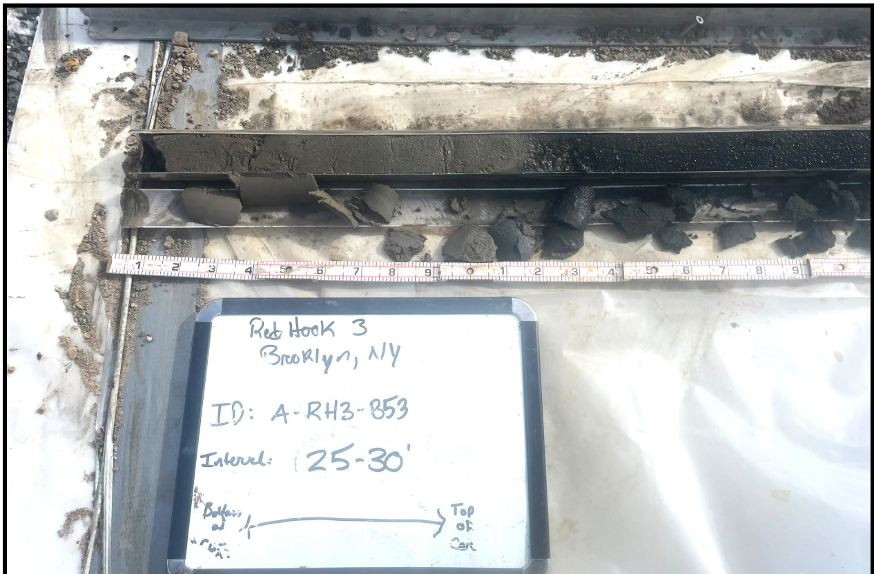
Photo 74: A-RH3-B53 – staining to 28.7 feet
