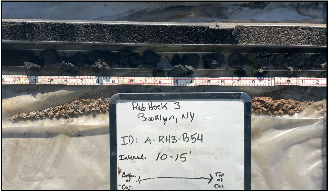
Photo 77: A-RH3-B54 – staining starting at 12.4 feet
