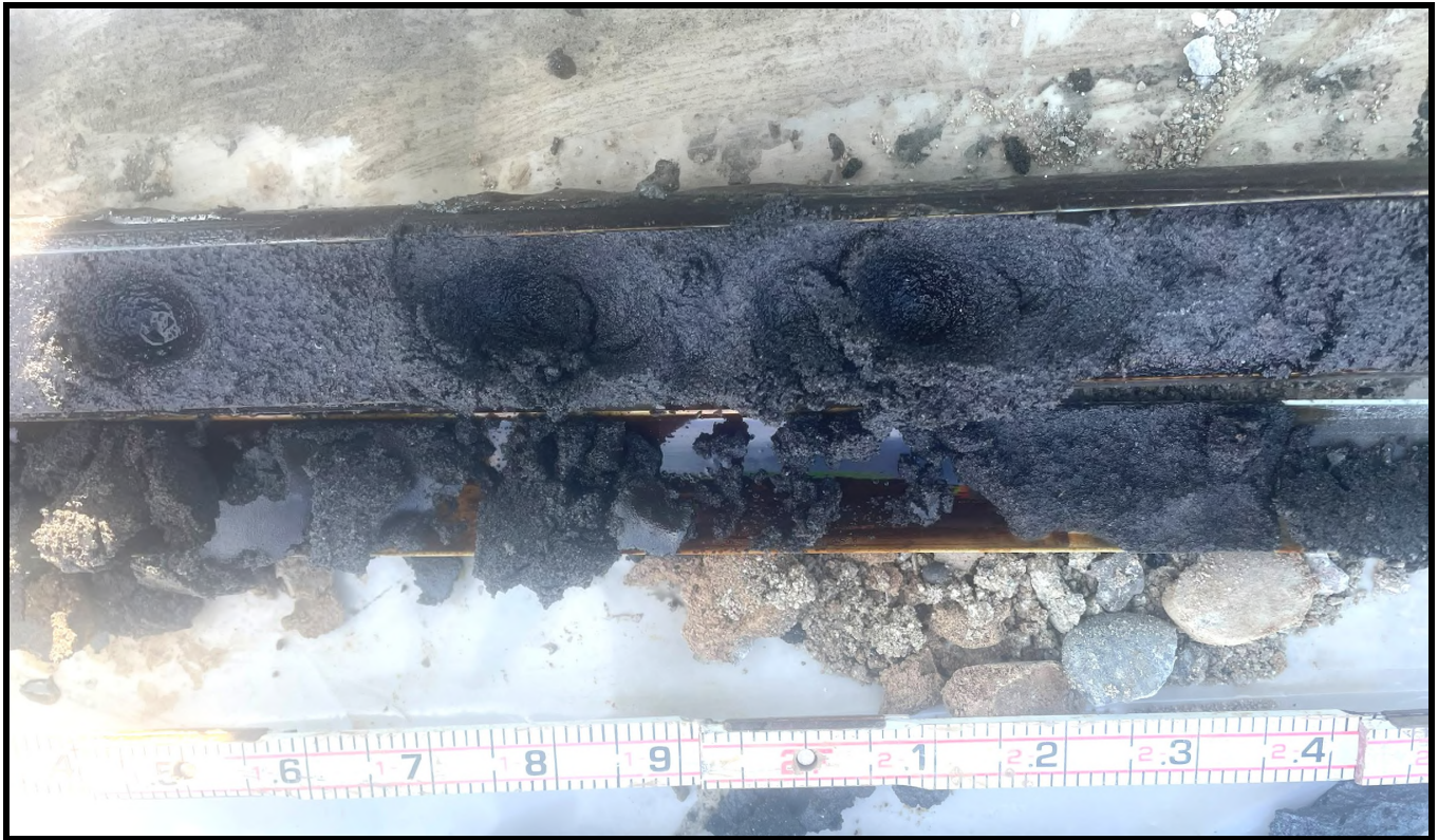
Photo 54: A-RH3-B51 – heavy staining and blebs at 18 feet
