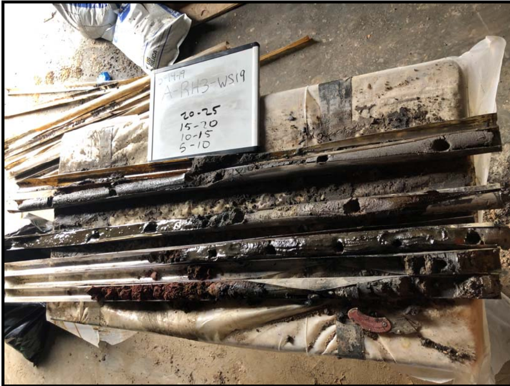
A-RH3-WS19: 5- to 25-Foot Soil Cores Showing Staining 11 to 17 Feet
