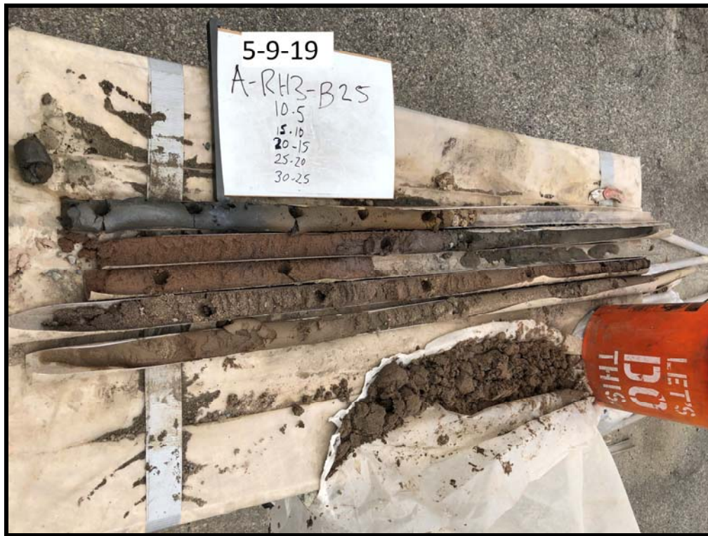
A-RH3-B25: Staining at 7 to 12 Feet
