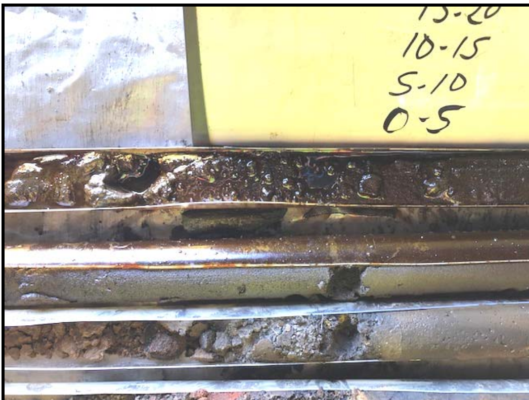
A-RH3-WS22: Close-up of NAPL at 20 to 21 Feet (Upper Sleeve)
