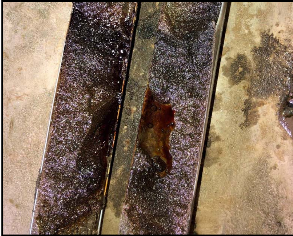
A-RH3-WS15: Close-up of NAPL in 23- to 24-Foot Interval
