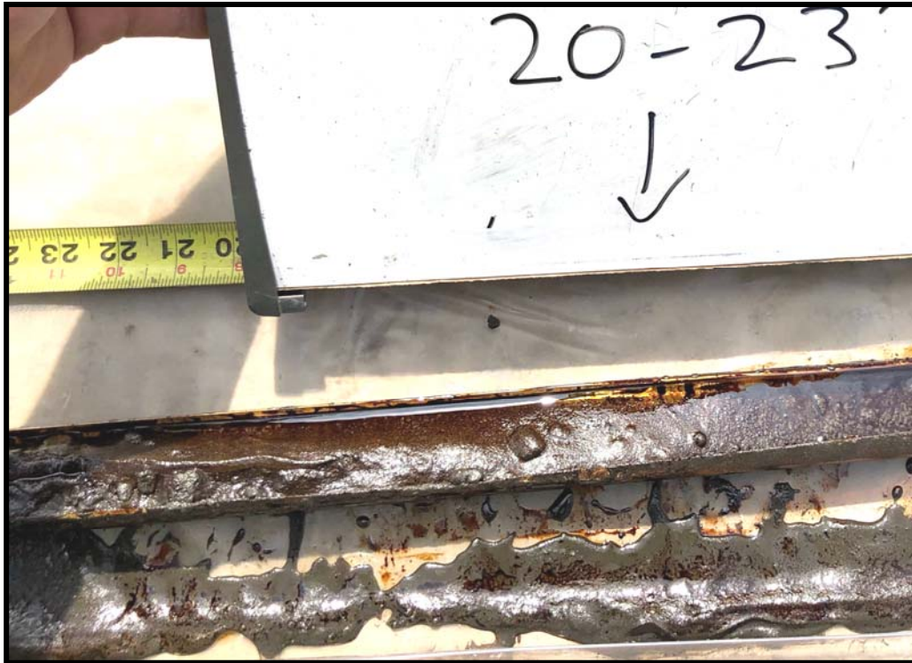
A-RH3-B39: Close-up of NAPL in 20- to 23-Foot Interval
