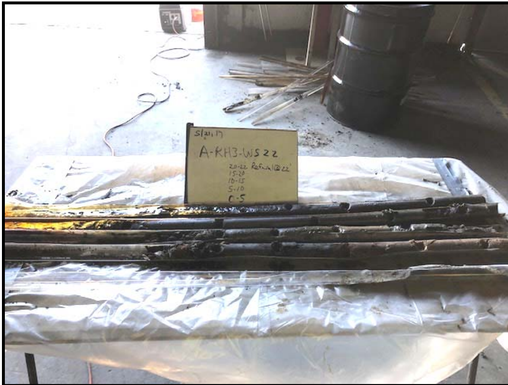
A-RH3-WS22: 0- to 25-Foot Soil Cores (Refusal at 22 Feet)
