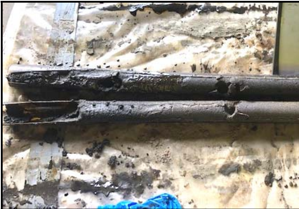
A-RH3-WS26: Staining at 20 to 22 Feet (Lower Sleeve) and Blebs 25 to 28 Feet (Upper Sleeve)
