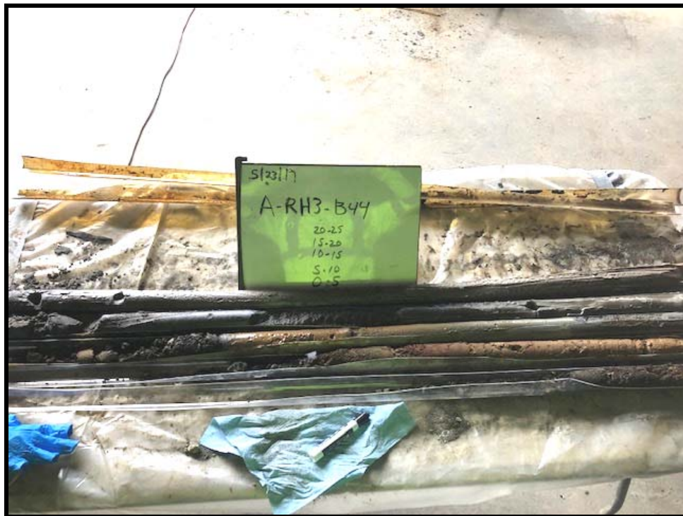
A-RH3-B44: 5- to 25-Foot Soil Cores (Refusal at 25 Feet)
