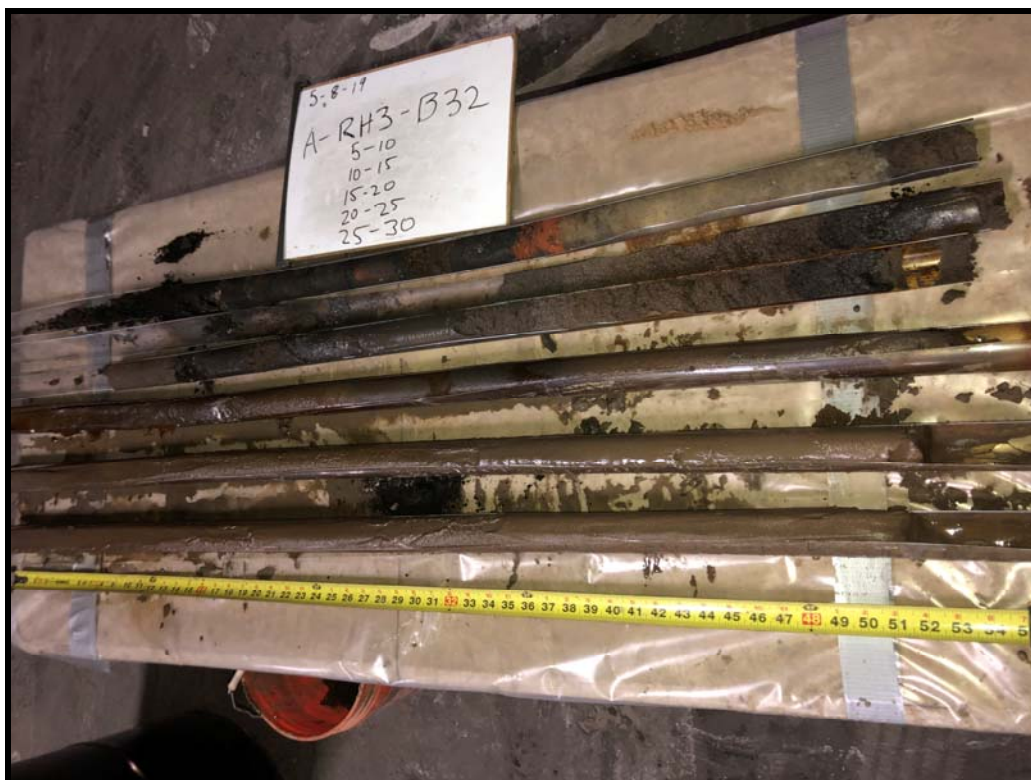
A-RH3-B32: 5- to 30-Foot Soil Cores
