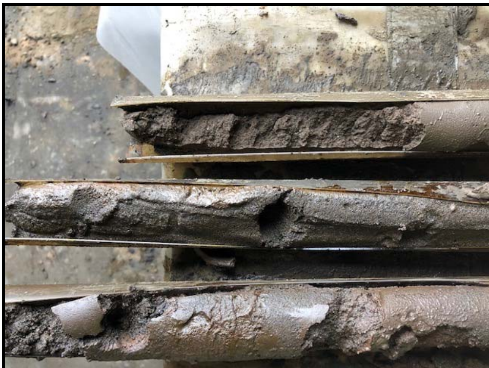
A-RH3-B41: Staining at 20 to 21 Feet
