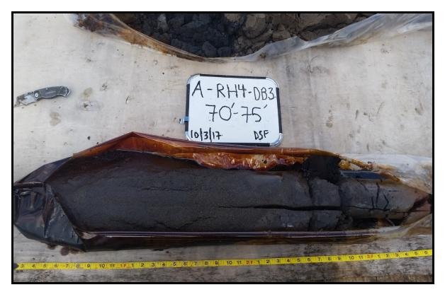
Soil core showing DNAPL saturation
