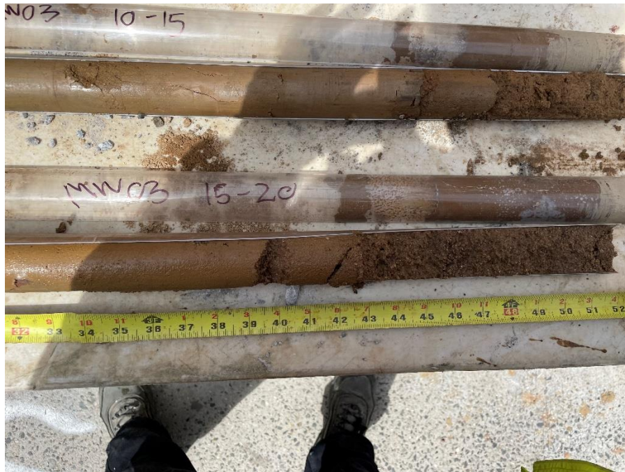
Photograph 3: MW03 macrocores from 10 to 20 feet below grade surface (bgs).
