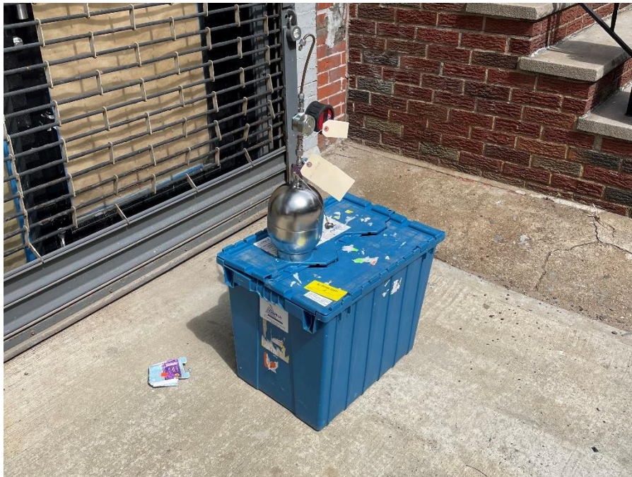
Photograph 6: Ambient air sample collection in the southeast part of the site (facing north).
