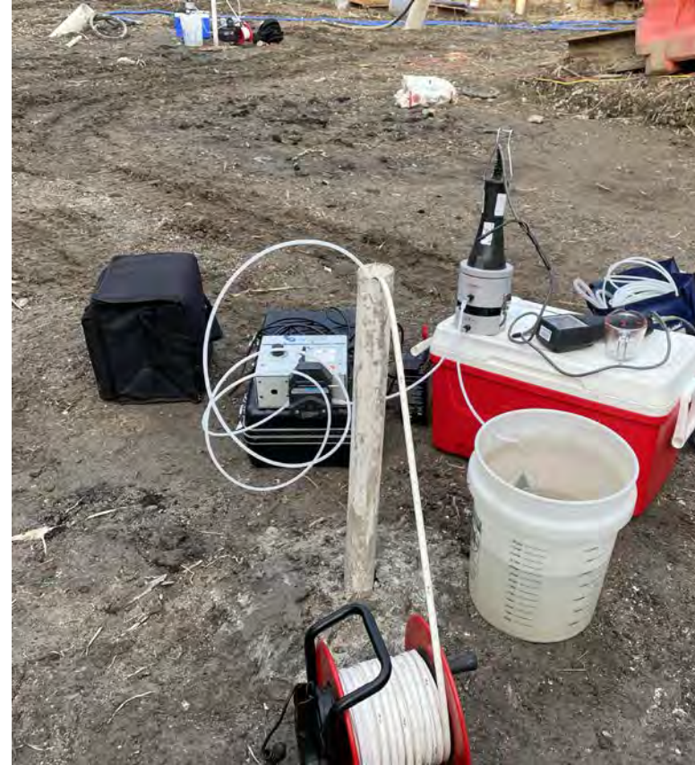
Photo 2: View of low flow purging at MW-01.
