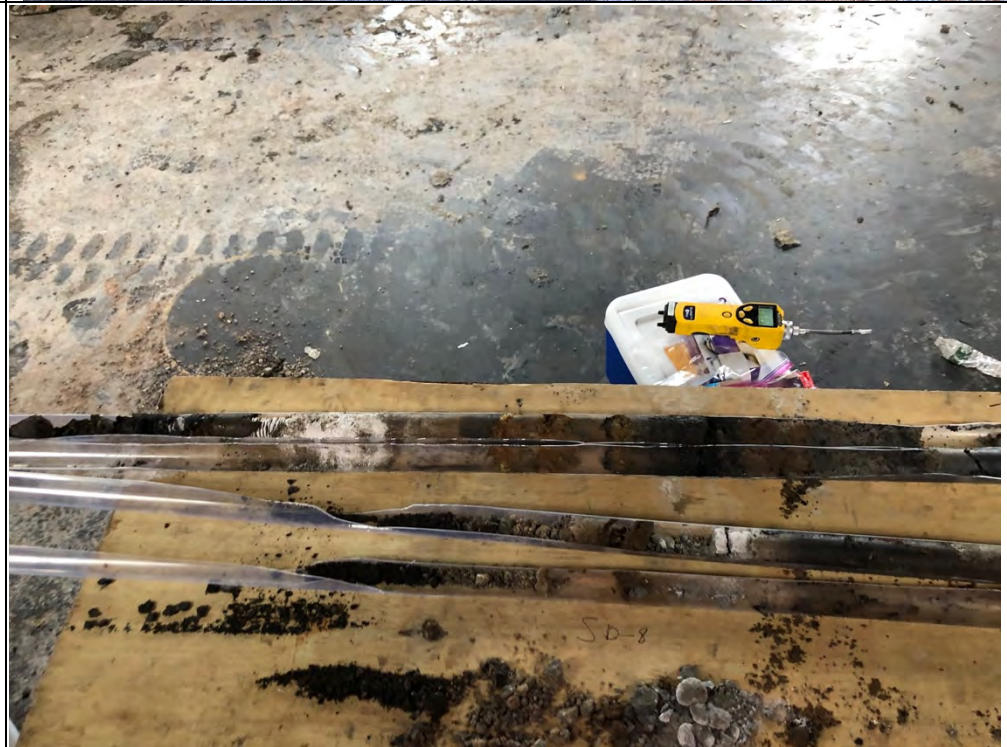
Photo 6: View of typical sleeves and soil samples (23B-8)
