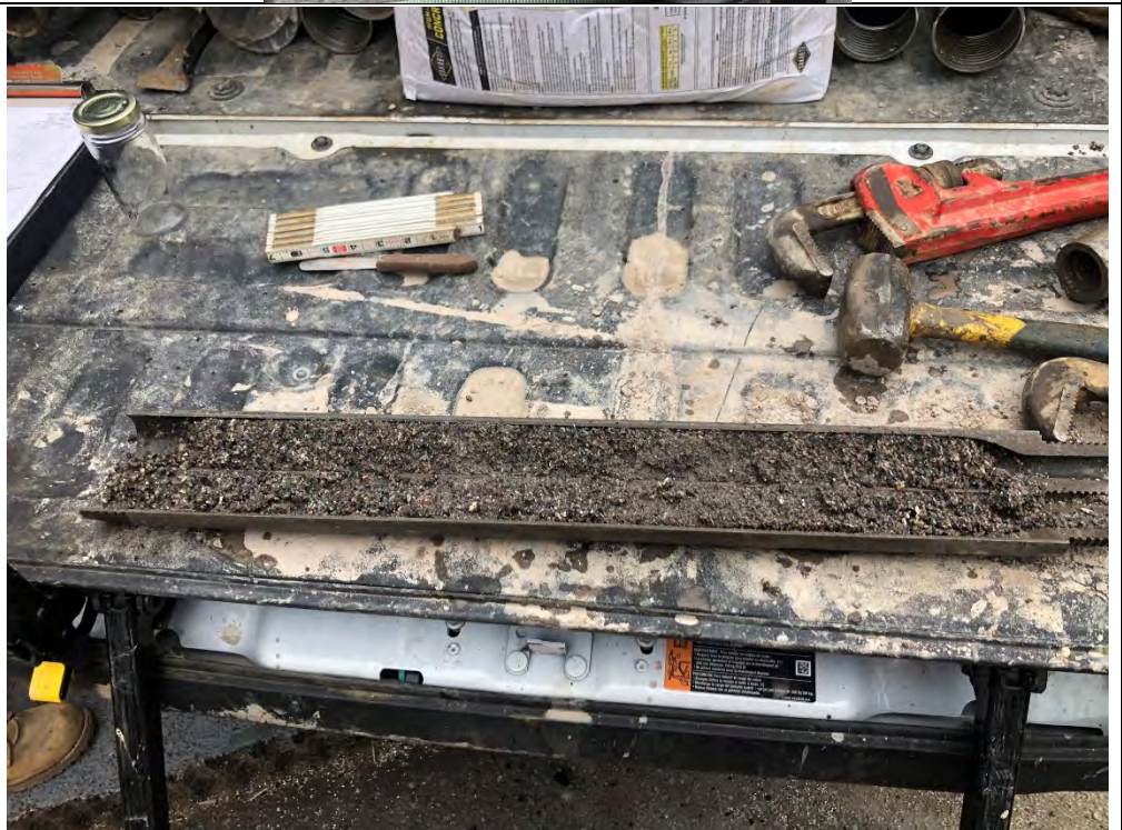
Photo 2: View of spoon sample from MR-12 collected at 65 feet bgs.
