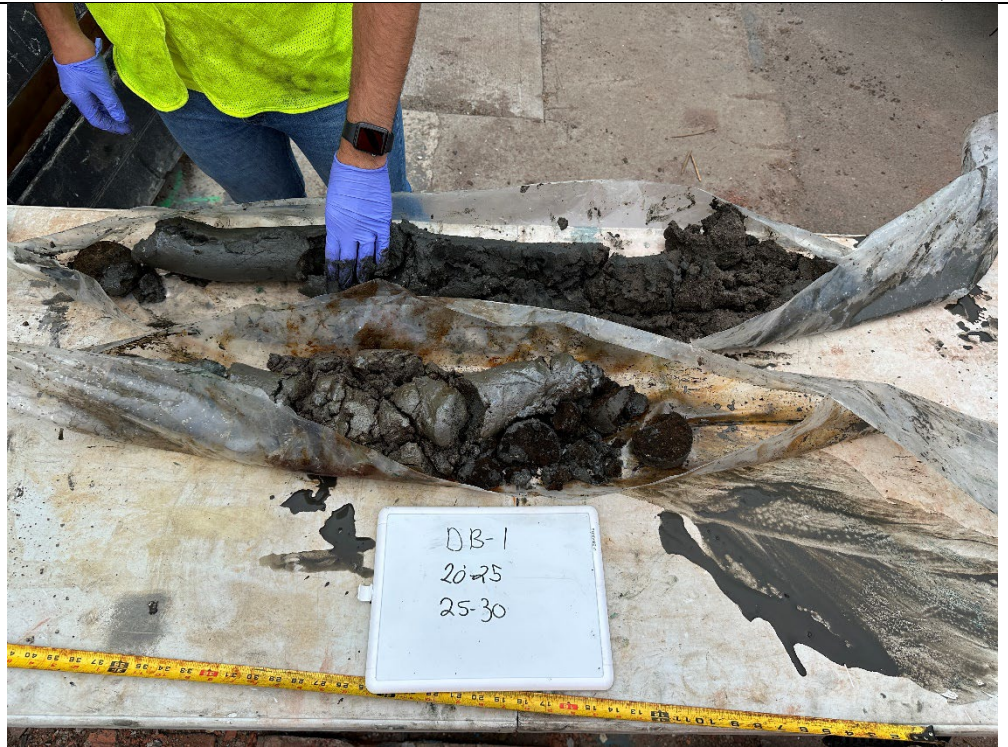
Photo 3: View of DB-1 sonic sleeves 20 to 25 feet and 25 to 30 feet. Coating and staining of coal tar is visible.
