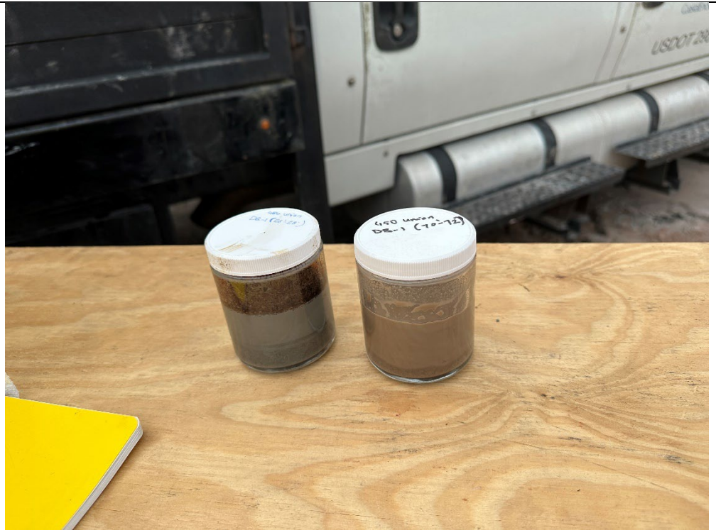
Photo 4: View of shake tests performed on DB-1 26 to 28 feet and DB-1 70 to 72 feet.
