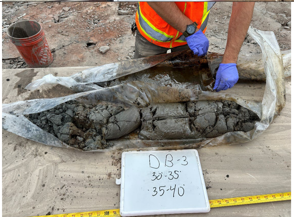
Photo 4: View of DB-3 sonic sleeves 30 to 35 feet and 35 to 40 feet. Coating and staining of coal tar is visible.
