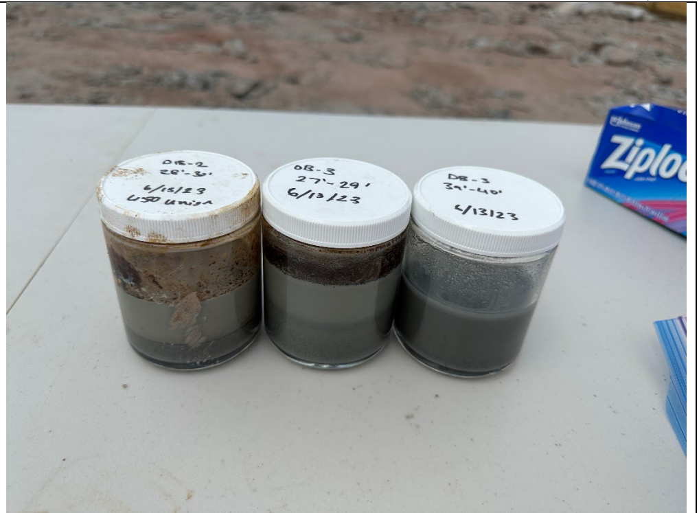
Photo 4: View of shake tests performed on DB-2 28 to 30 feet, DB-3 27 to 29 feet, and DB-3 39 to 40 feet.
