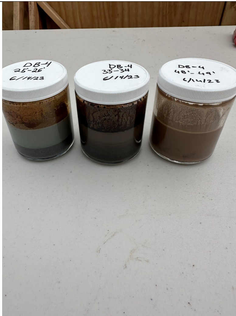
Photo 4: View of shake tests from DB-4 from intervals 25-26 feet, 33-34 feet, and 48-49 feet.
