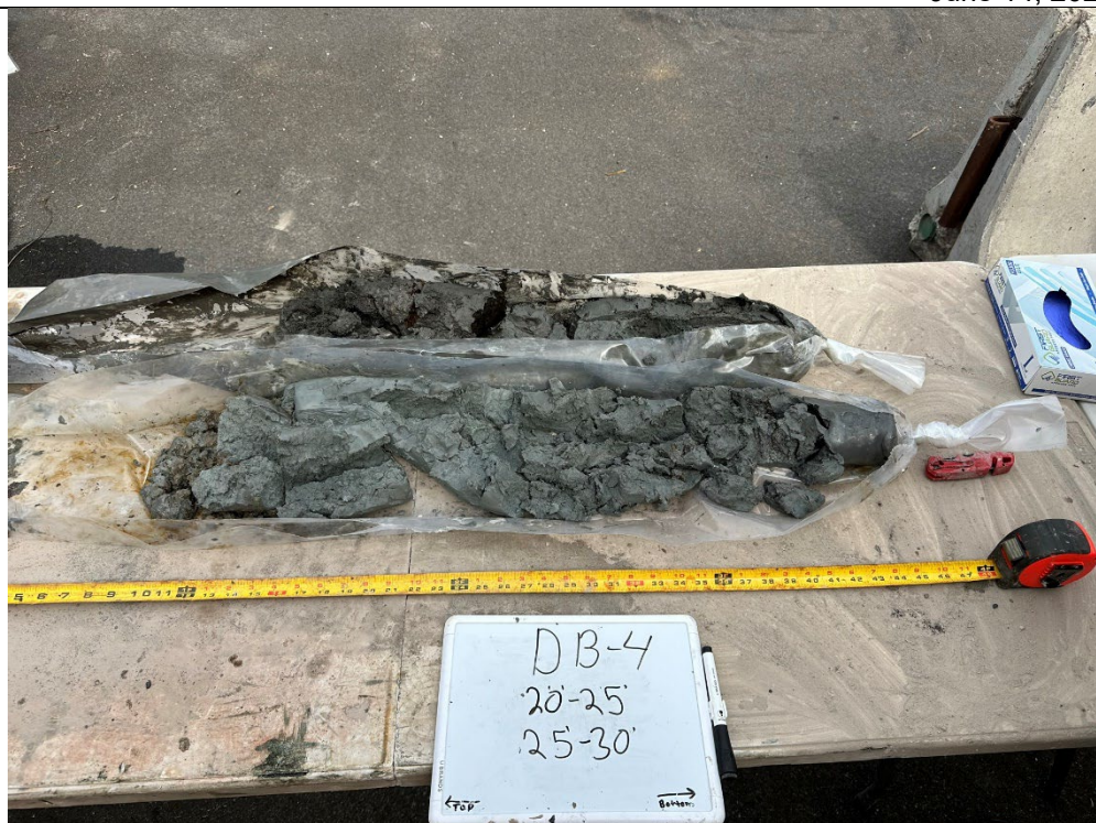
Photo 3: View of DB-4 sonic sleeves 20 to 25 feet and 25 to 30 feet.
