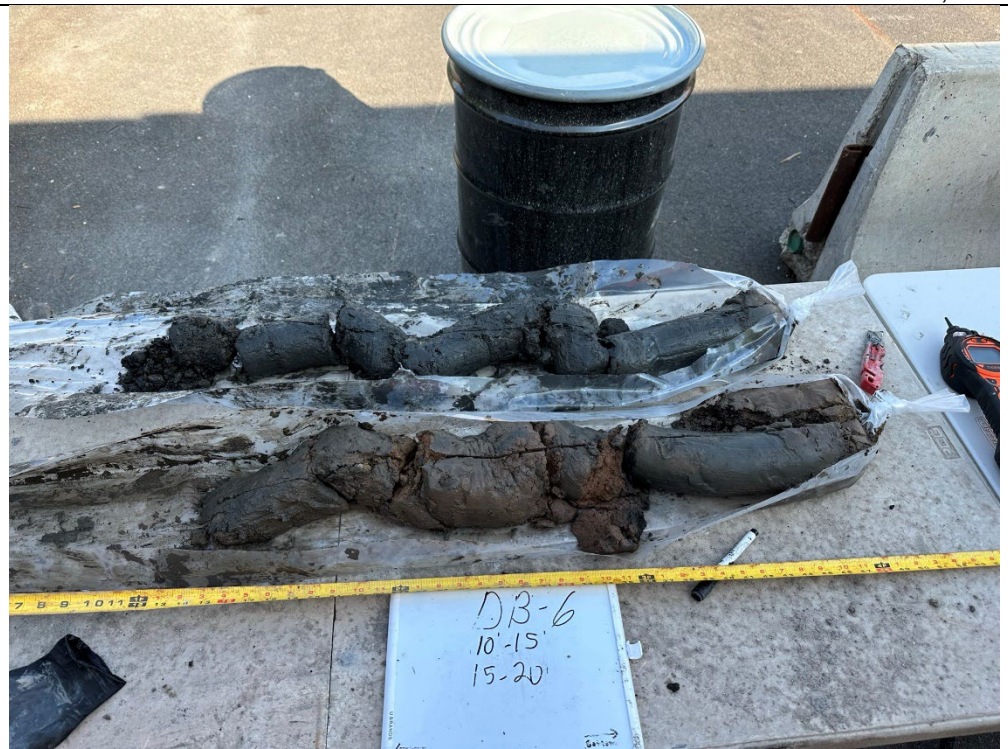
Photo 2: View of DB-6 sonic sleeves 10 to 15 feet bgs. and 15 to 20 feet bgs.
