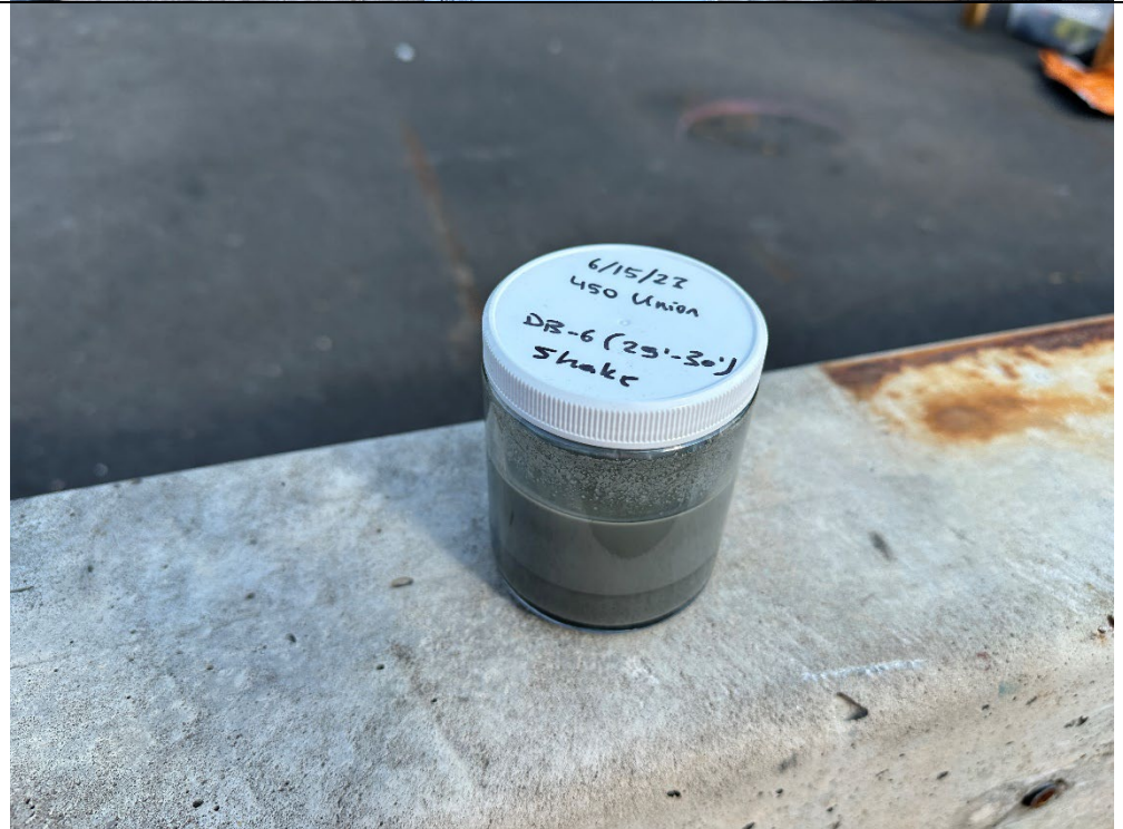
Photo 3: View of shake test from DB-6 29 to 30 feet bgs.
