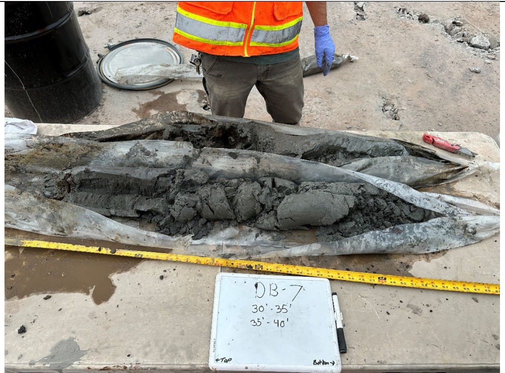
Photo 4: View of DB-7 sonic sleeves 30 to 35 feet and 35 to 40 feet.
