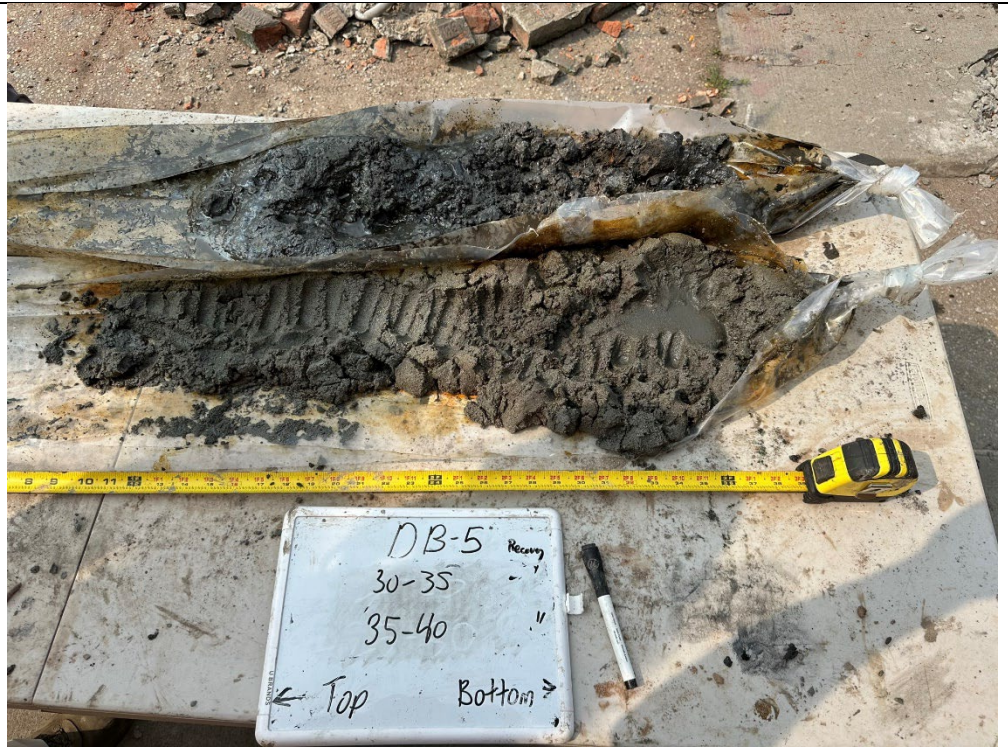
Photo 4: View of DB-5 sonic sleeves 30 to 35 feet and 35 to 40 feet. GMC evidence throughout both sleeves.
