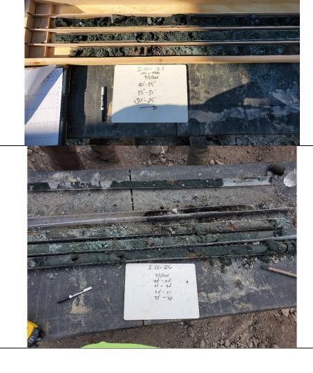
Photo 4: View of confirmation cores from ISS-3C from 20 to 35 feet for visual inspection.
