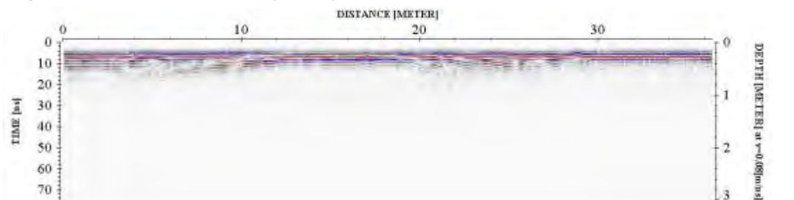
**Step 3.** Correct for attenuation losses (*energy decay function*)
