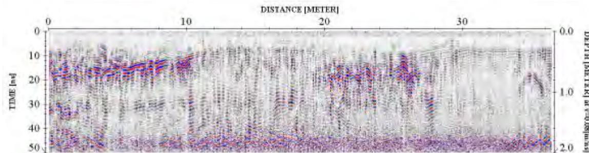
The above example shows the significance of data processing. The last image (step 5) has higher resolution than the starting image (raw data – step 1) and describes the subsurface anomalies more accurately.
