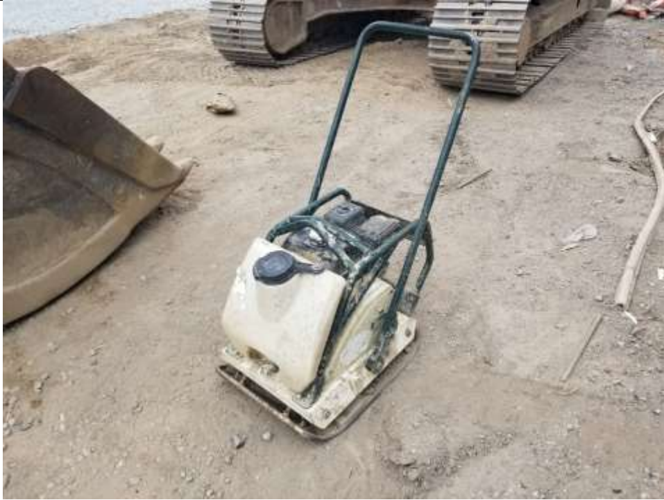
Photo 3: View of Sakai PC800 plate tamper used for compaction activities.
