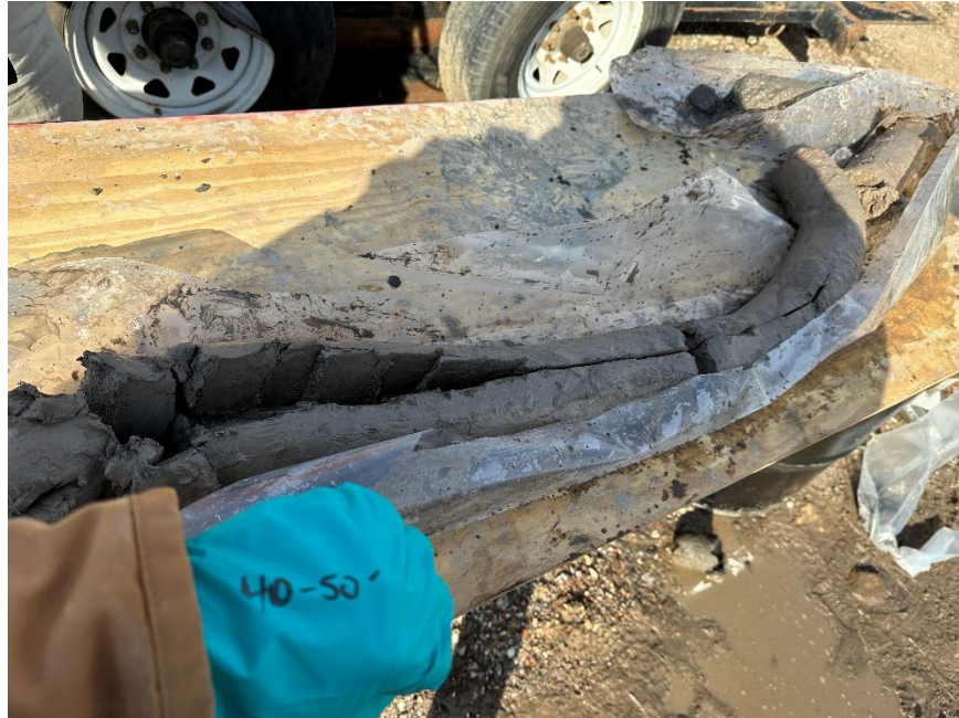
Photo 2: View of soil/fill recovered from soil boring SSB-02 (facing north)
