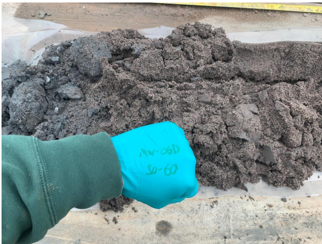
Photo 2: View of recovered soil from 50 to 60 feet bgs during installation of monitoring well SMW-06DGD (facing north)
