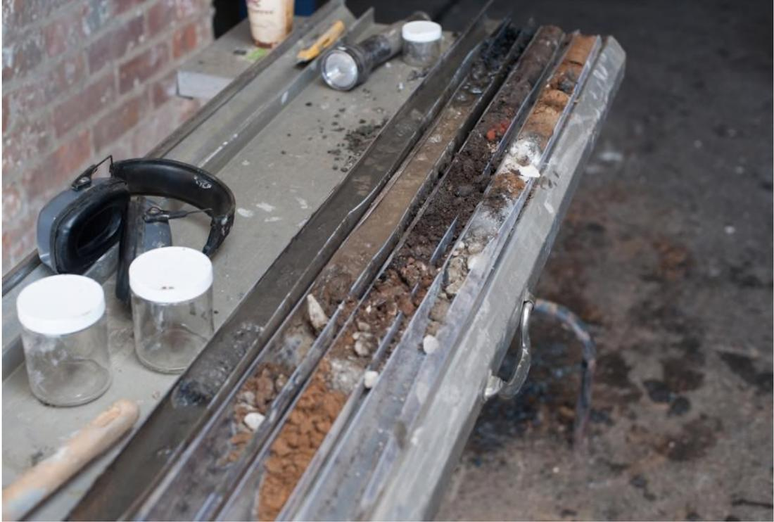
**Photograph 3:** Typical fill material encountered in the borings (B3 shown)
