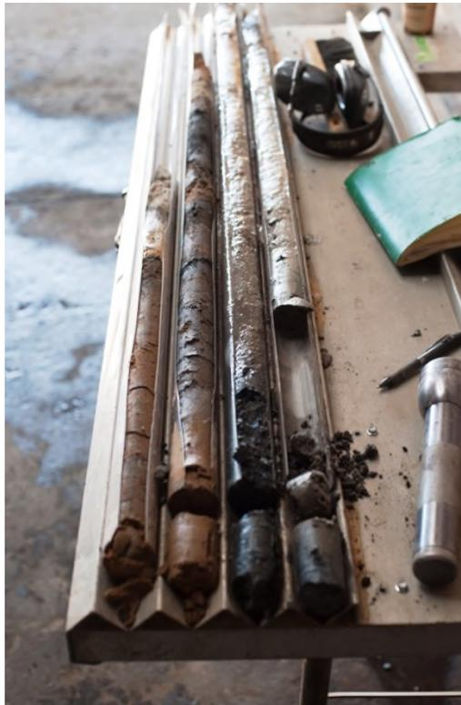
**Photograph 4:** Discolored soil at water table (black material) shown in samples from B3.
