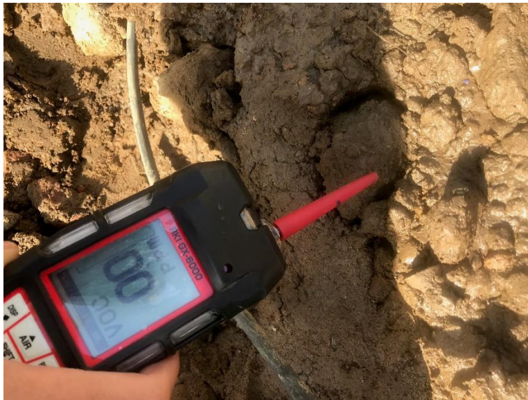
Photo 22: Screening of non-hazardous historic fill material within the encountered 550-gallon UST grave; evidence of impacts were not observed. Taken on 03/21/2020.
