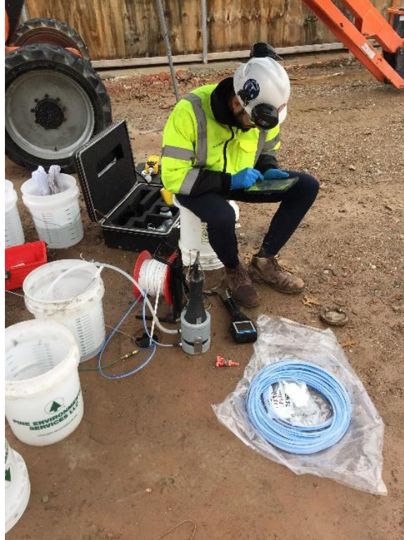
Photo 5: Langan conducting post-injection low-flow groundwater sampling of monitoring well MW-111 (facing south). Taken on 12/10/2019.
