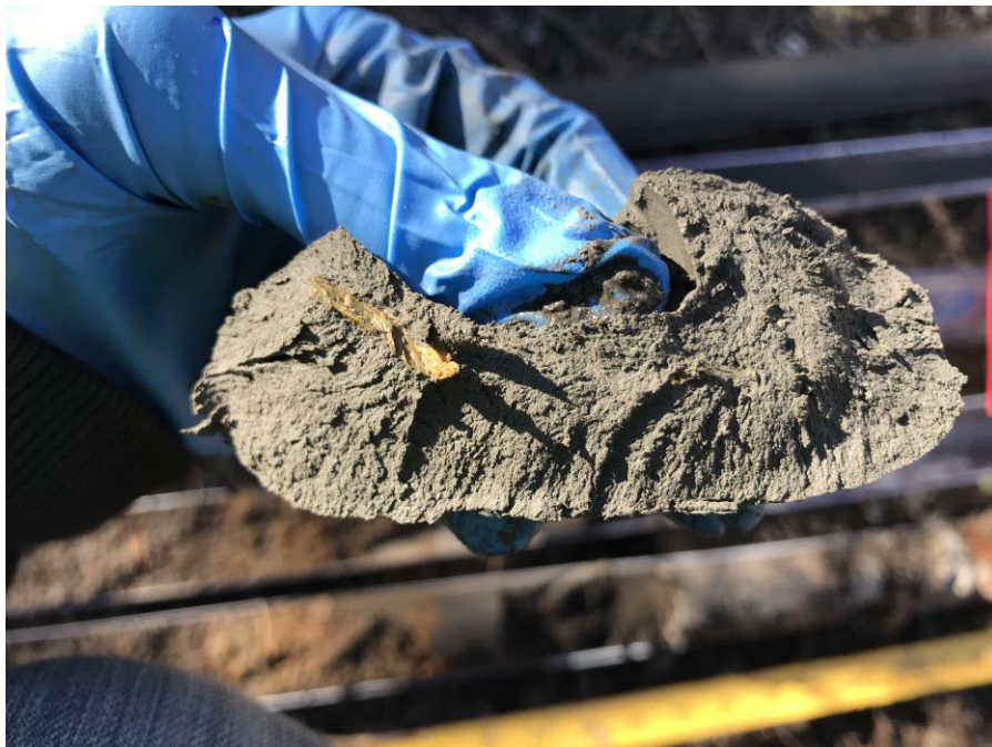
Photo 10, 11/21/2017: Clay interval observed at about 15' bgs within soil boring 16MW2, facing down.
