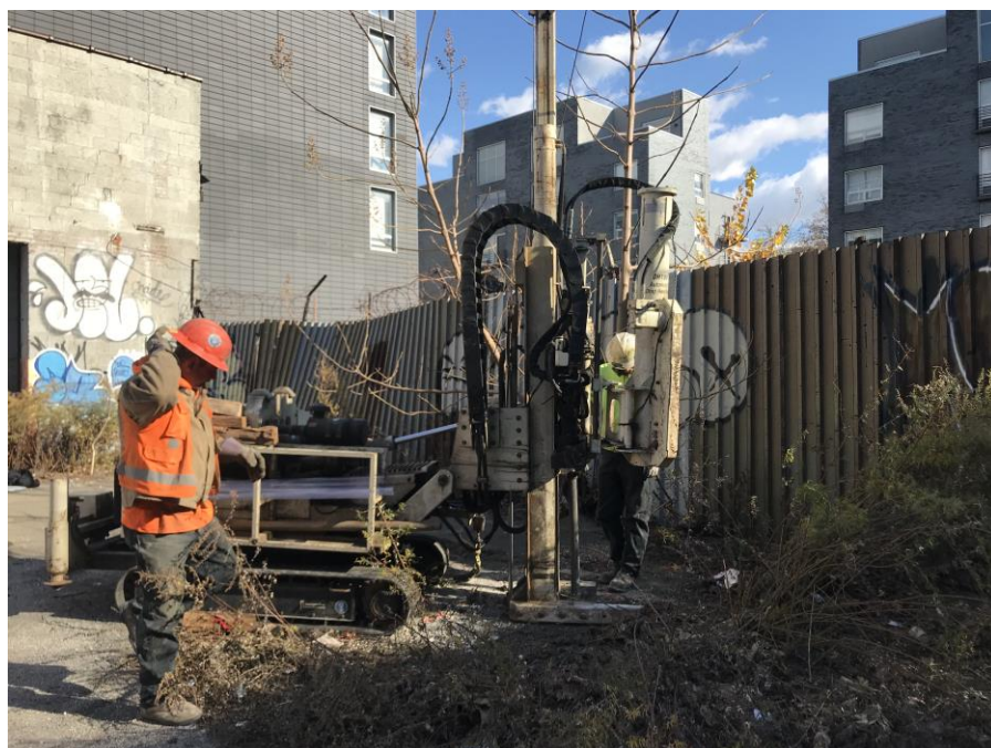
Photo 6, 11/20/2017: AARCO advancing soil boring 16B5 using a Geoprobe 6610DT, facing east.
