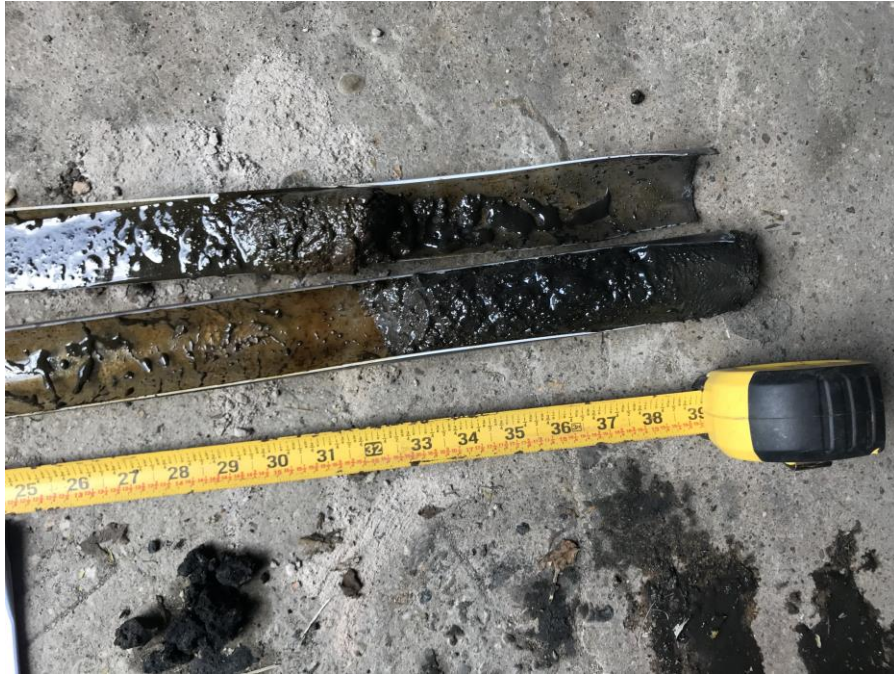
Photo 3, 11/20/2017: Soil recovery and product observed within soil boring 16B1 (8 to 12 feet bgs), facing down.
