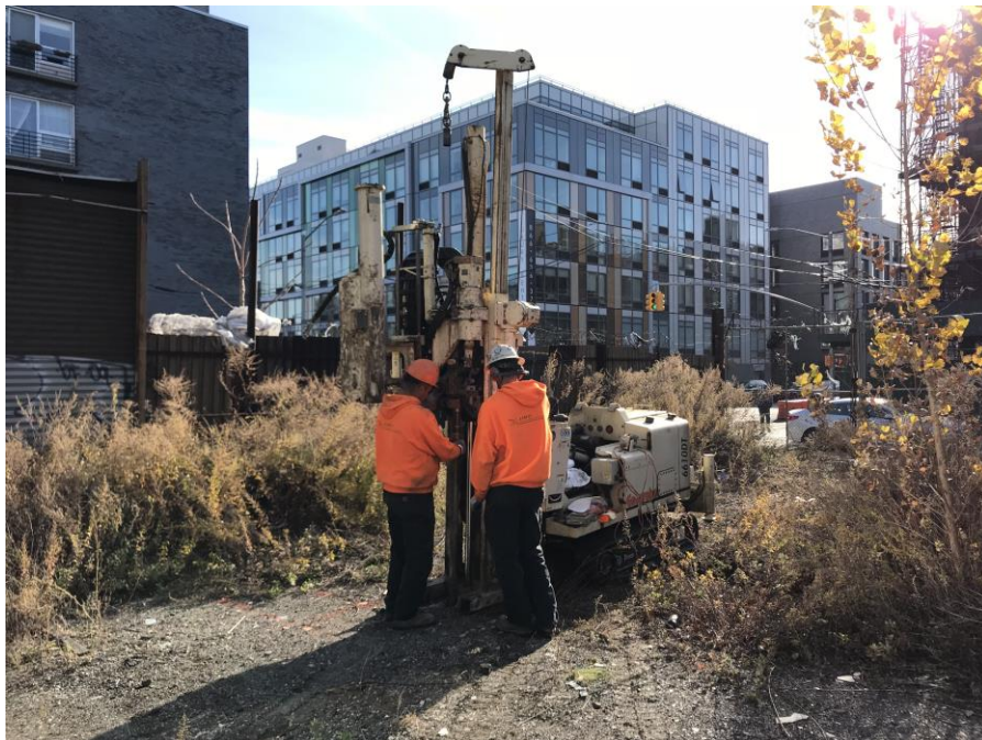
Photo 12, 11/21/2017: AARCO advancing soil boring 16B4 using a Geoprobe 6610DT, facing south.
