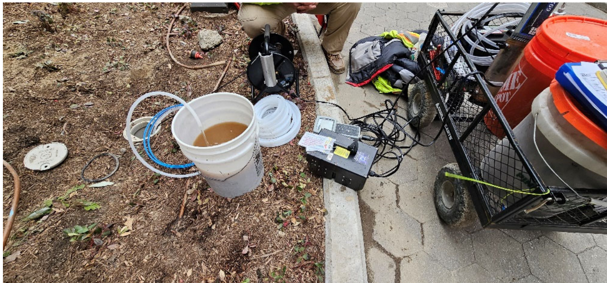
10 – Purging a monitoring well as part of the post-remedial groundwater sampling event.
