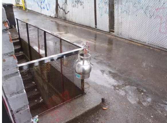
Outdoor ambient air sample AA-1 being collected at the west side of the retail space
