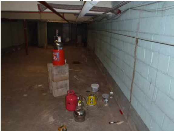
Indoor air (IA-1) and sub-slab soil gas (SS-1) samples being collected
