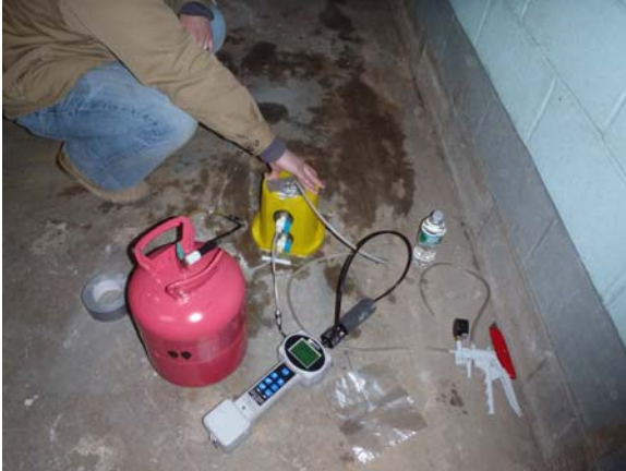
Tracer gas test being performed
