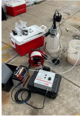
Photo 1: View of low flow sampling set up.
