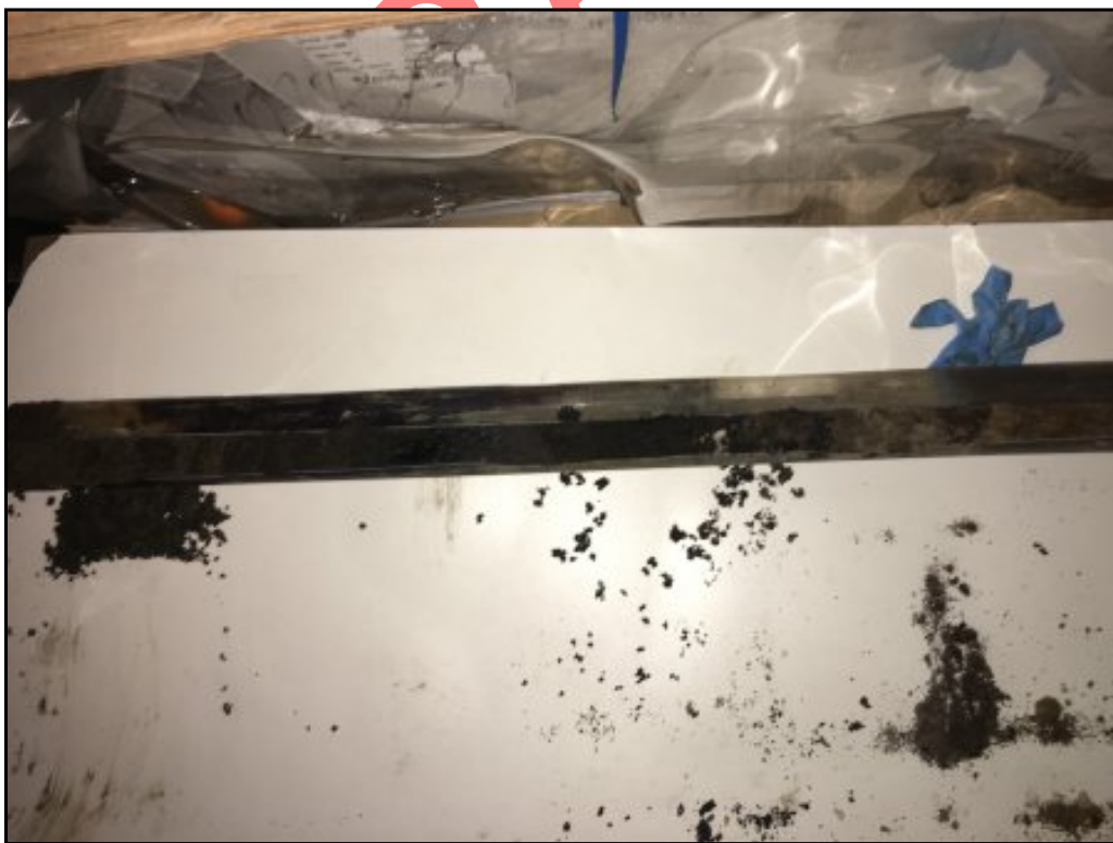
18 : Soil borings during TPH sampling - staining noted
