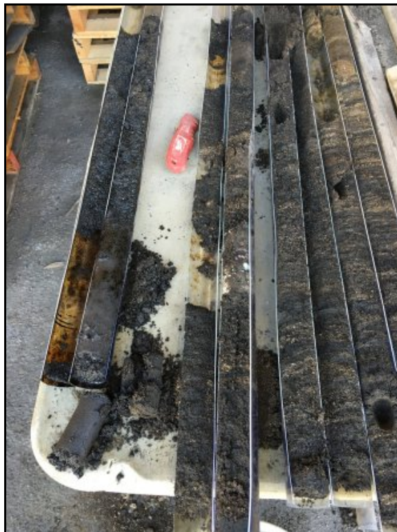
11 : Heavy staining borings
