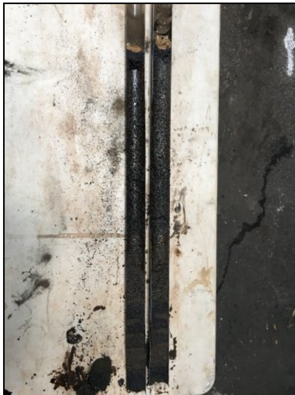
19 : Soil borings during TPH sampling - staining noted
