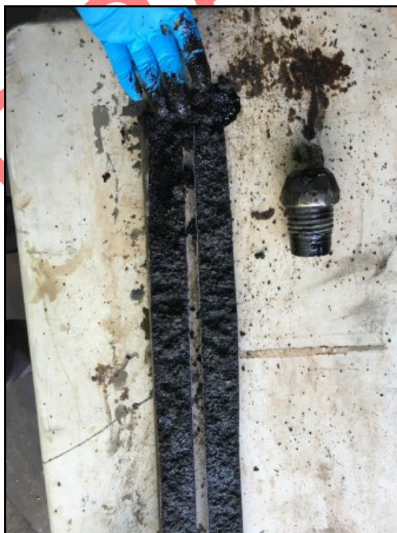
20 : Soil borings during TPH sampling - heavy staining noted
