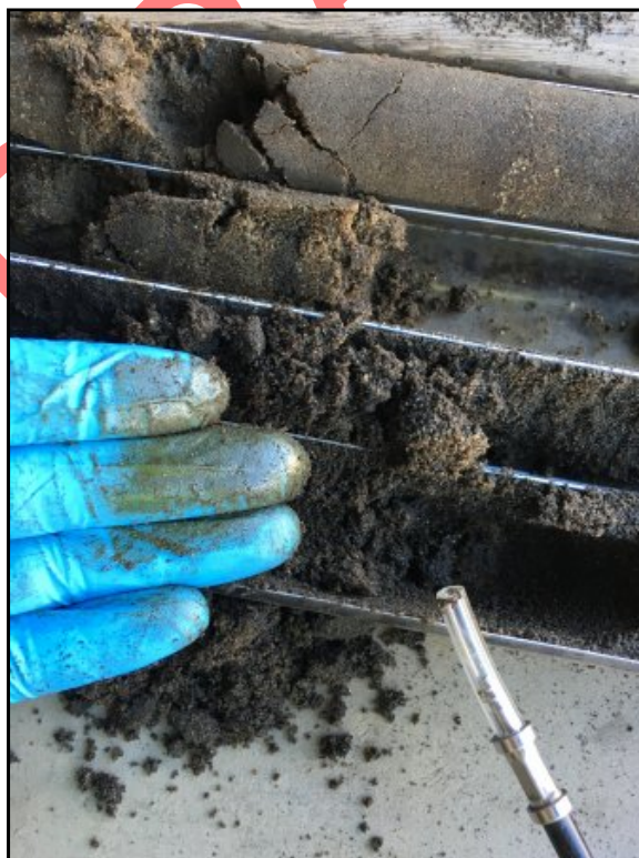
10 : Stained soil boring
