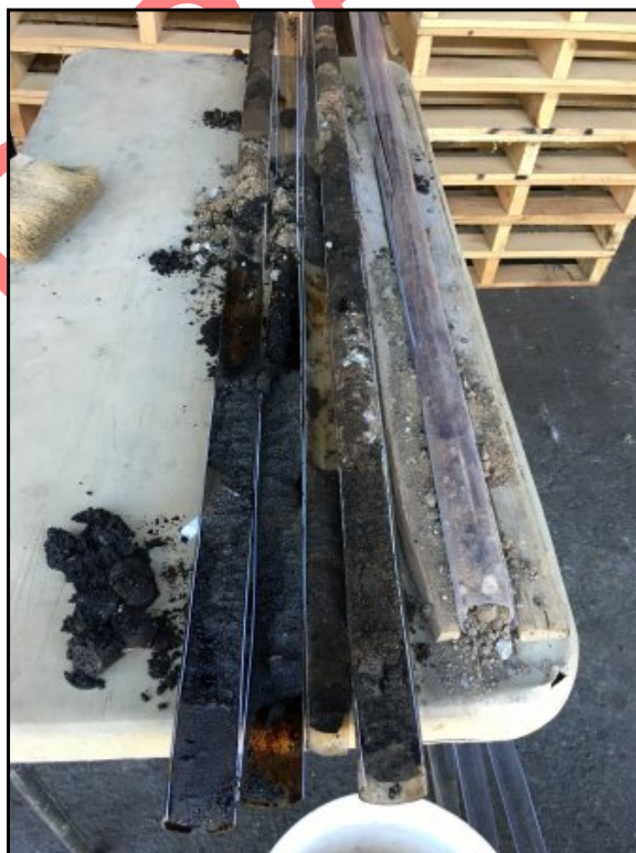
6 : View of soil borings with petroleum impacts
