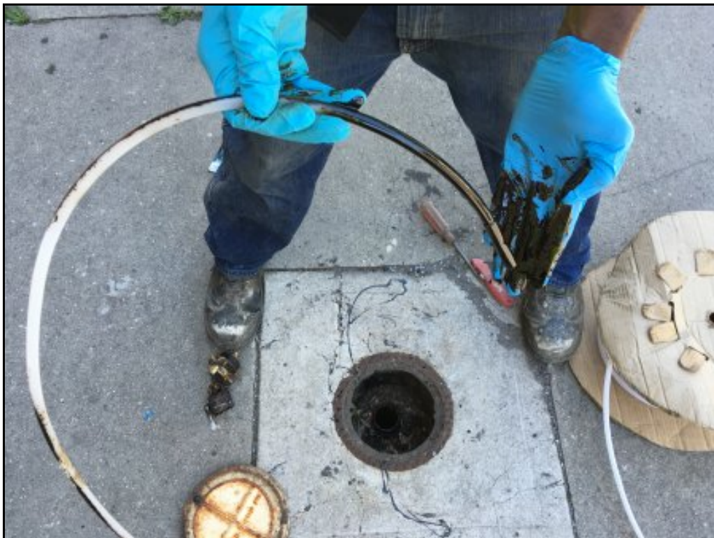
5 : View of noted "free product" in monitoring well on Barbey Street
