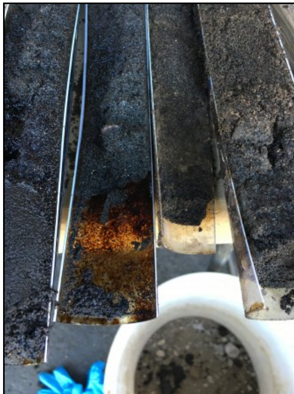
7 : View of soil borings with petroleum impacts
