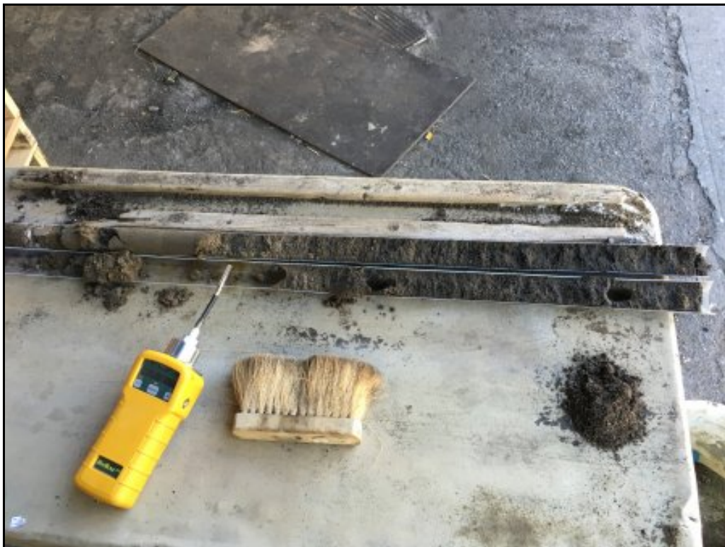
9 : PID screening soil boring
