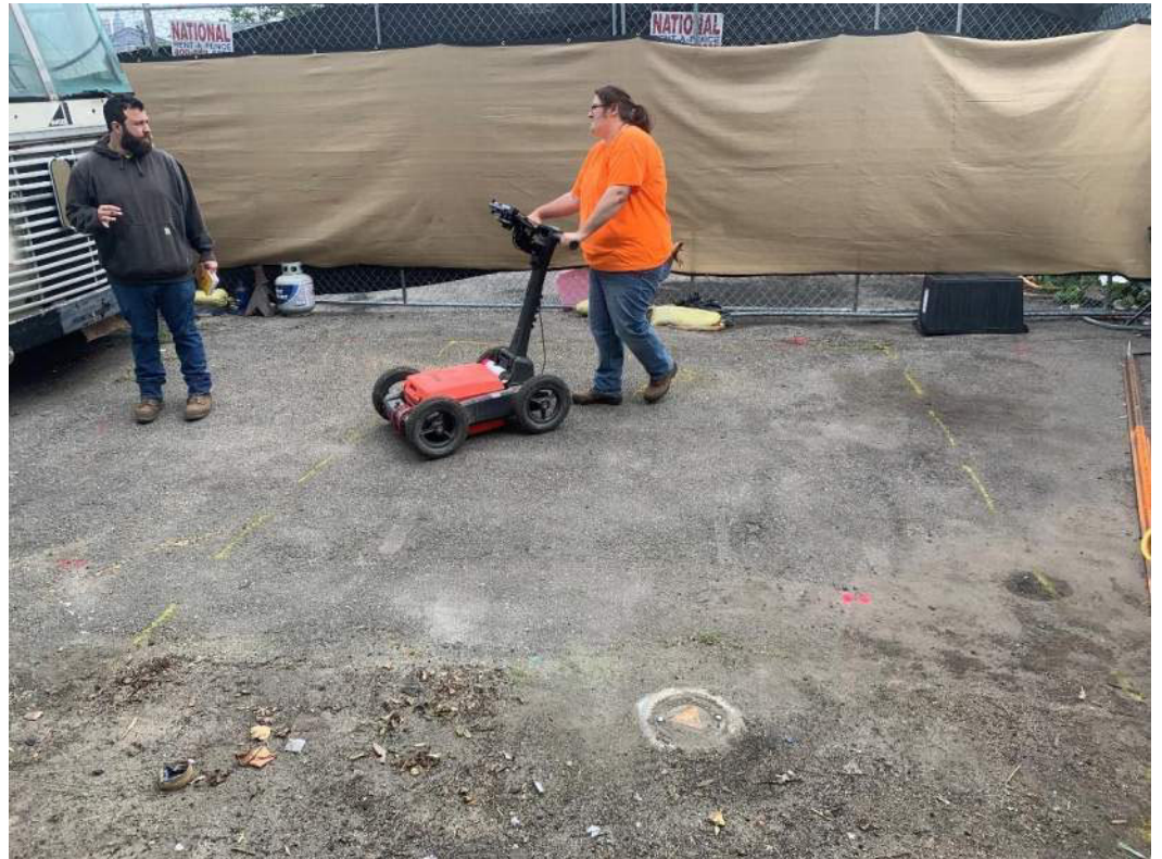
Photo 3: View of Hager Richter performing Geophysical Survey around TP-02.
