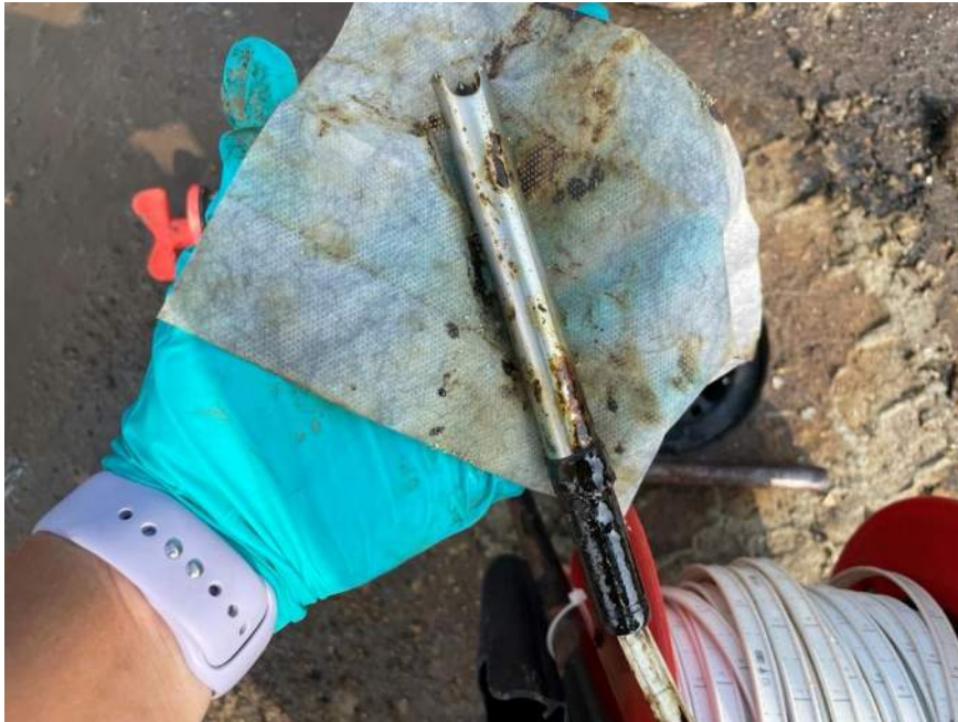
Photo 1: LNAPL encountered within monitoring well MW-03D.
