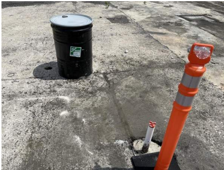
Photo 2: Groundwater monitoring well MW07 and a 55-gallon drum containing IDW (soil cuttings)
