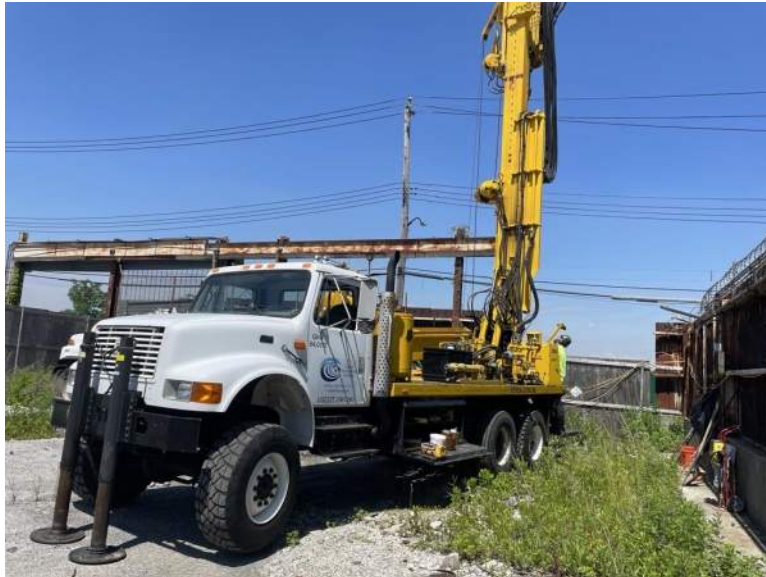
Photo 1: Coastal advancing soil boring SB01 in the northern part of the site (facing north)
