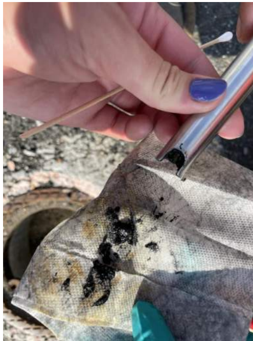
Photo 4: Viscous, black, immiscible liquid encountered within MW-008
