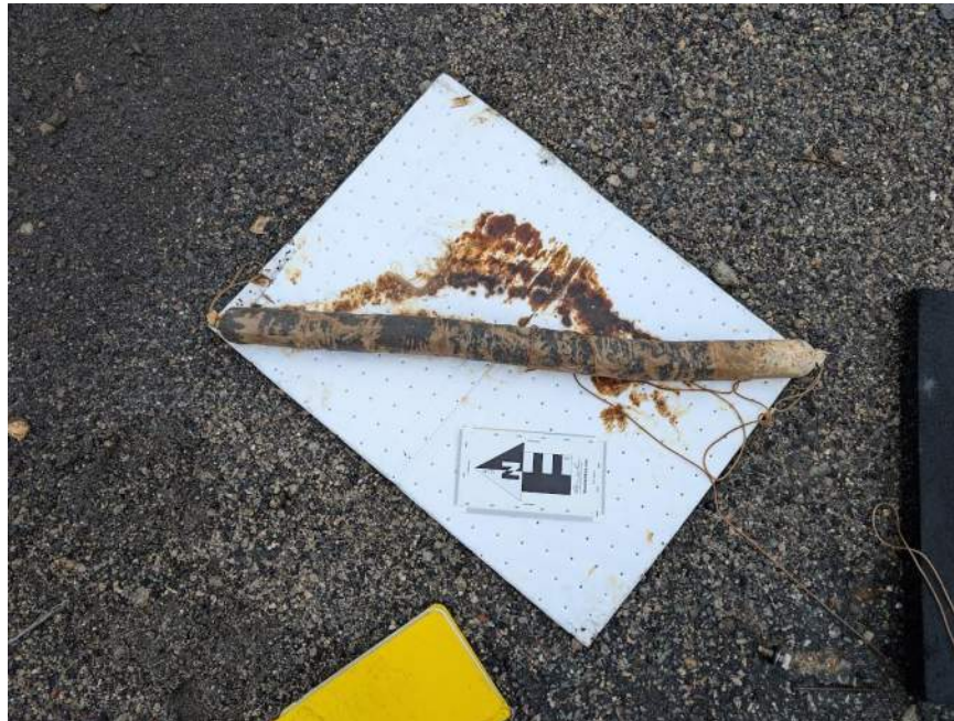
Photo 2: Oil absorbent sock removed from monitoring well MW-002.
