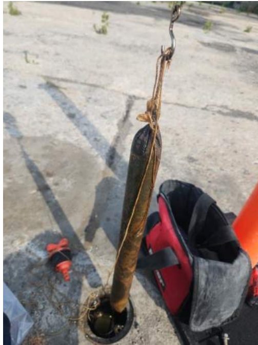
Photo 1: Absorbent sock removed from MW-012
