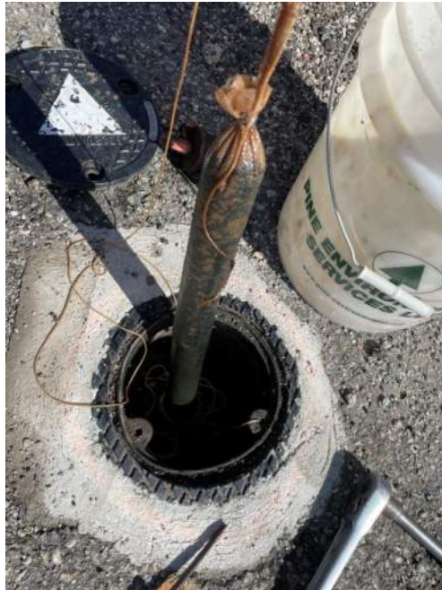
Photo 1: Absorbent sock removed from MW-002
