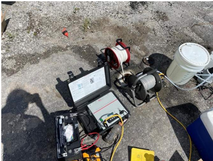
Photo 2: Langan purging groundwater from monitoring well MW-03D in the western part of the site.
