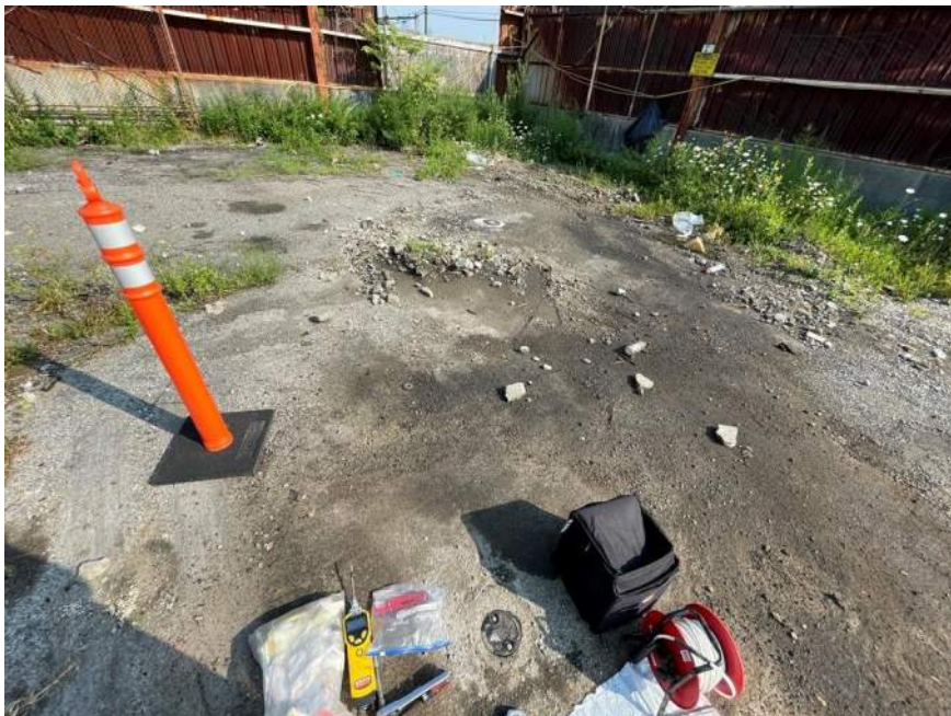
Photo 2: Langan gauging monitoring well MW-01D (facing north).
