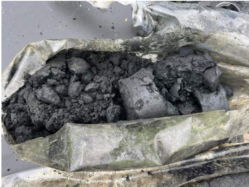
Photo 2: Recovered stained soil from about 5 to 10 feet bgs at SBD09.
