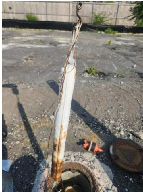
Photo 2: Absorbent sock removed from MW-014
