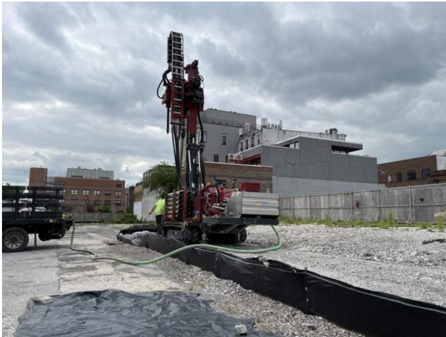
Photo 2: Coastal advancing soil boring SBD06 in the central part of the site (facing south)
