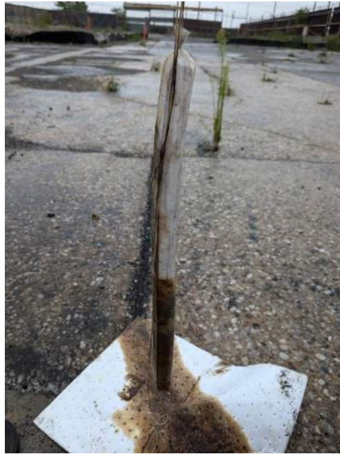
Photo 1: Oil absorbent sock removed from monitoring well MW-012.
