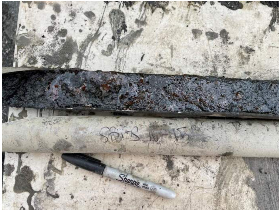
Photo 2: SBT-S soil boring core from 10 to 15 feet bgs with black tacky material and sheen
