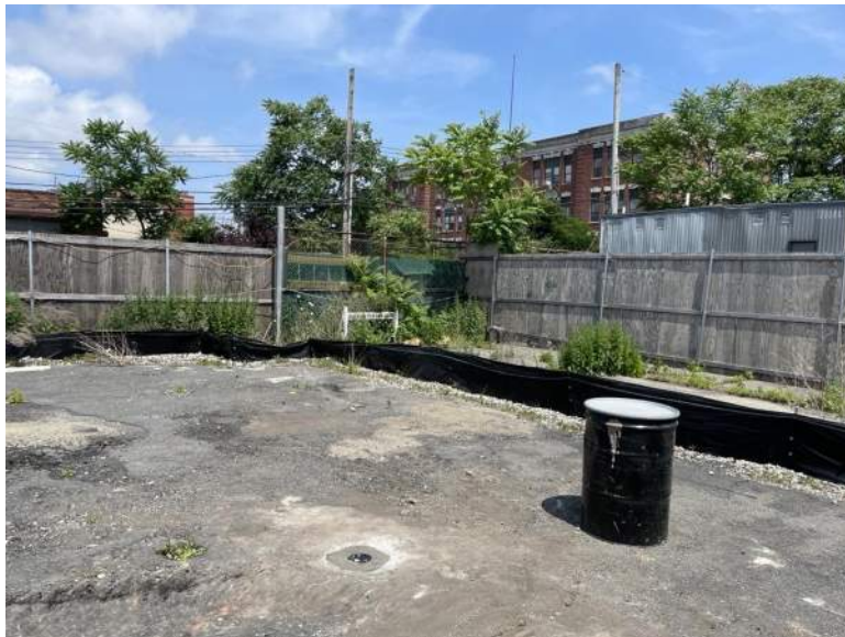
Photo 2: Groundwater monitoring well MW09 and a 55-gallon drum containing IDW (soil cuttings)
