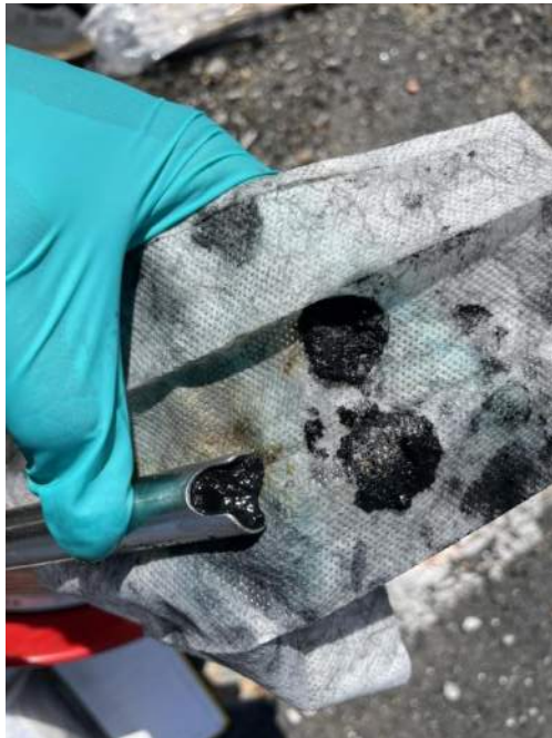
Photo 4: Viscous, black, immiscible liquid encountered within MW-008
