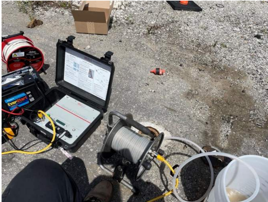
Photo 1: Langan purging groundwater from monitoring well MW-02D in the central part of the site.
