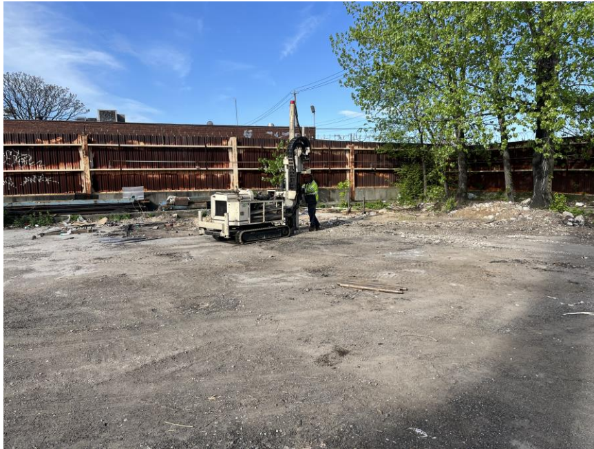
Photo 1: Eastern advancing soil boring WC11B_W10 in the northwestern part of the site (facing west)
