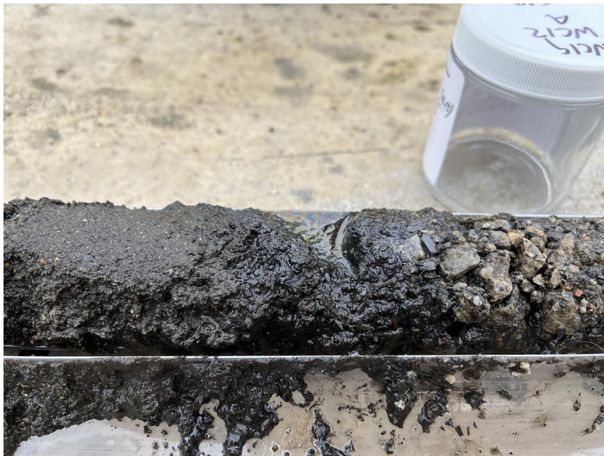
Photo 2: Soil boring core from 9 to 13 feet bgs at WC12A_S10
