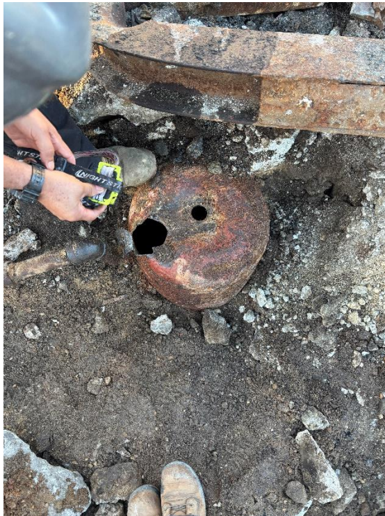
Photo 4: Suspect hydraulic oil tank observed in the eastern part of the site.
