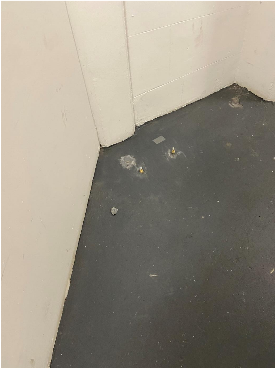
Photograph No. 1: View of typical sub-slab soil vapor monitoring point installation and duplicate sample location
