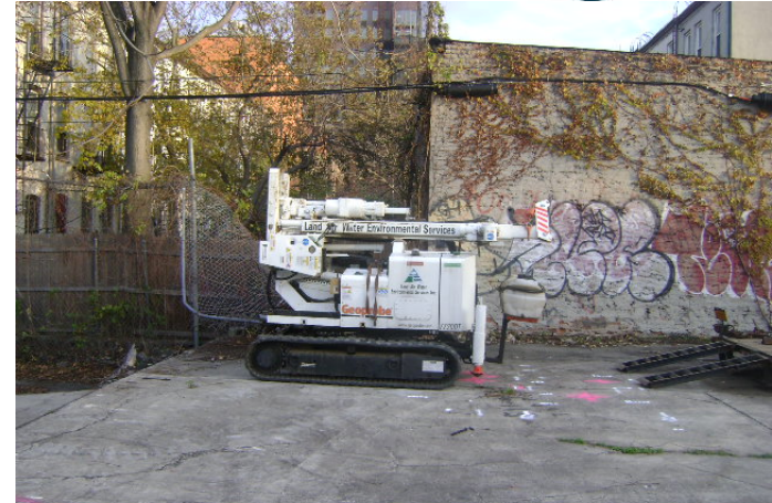
Photograph 6. View of Geoprobe set up to begin drilling at TRC-SB-4.
