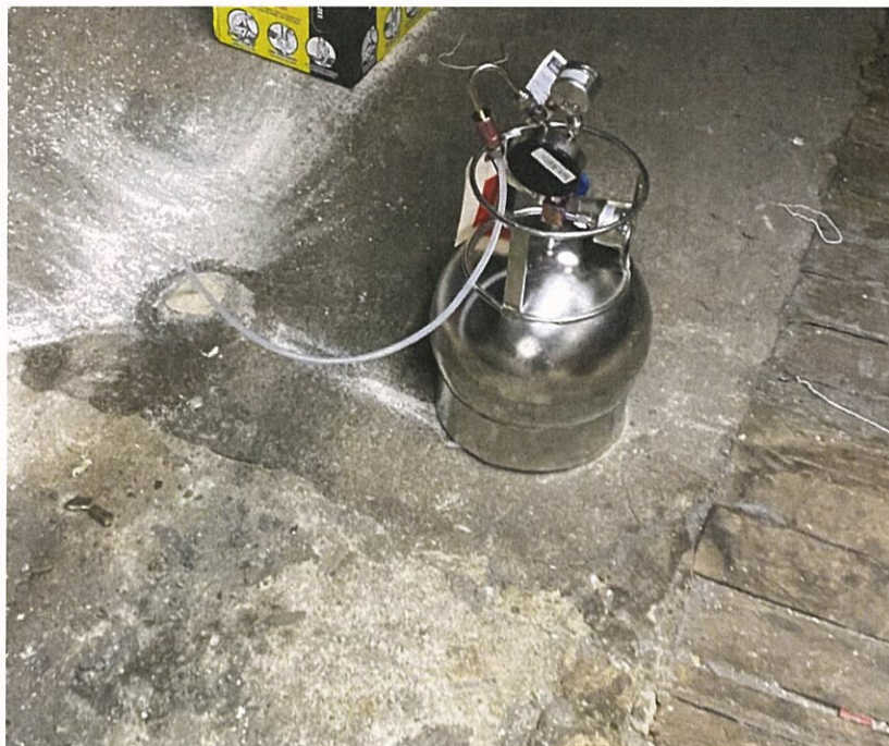
Image 2: View of an example of sub-slab vapor sampling equipment.
