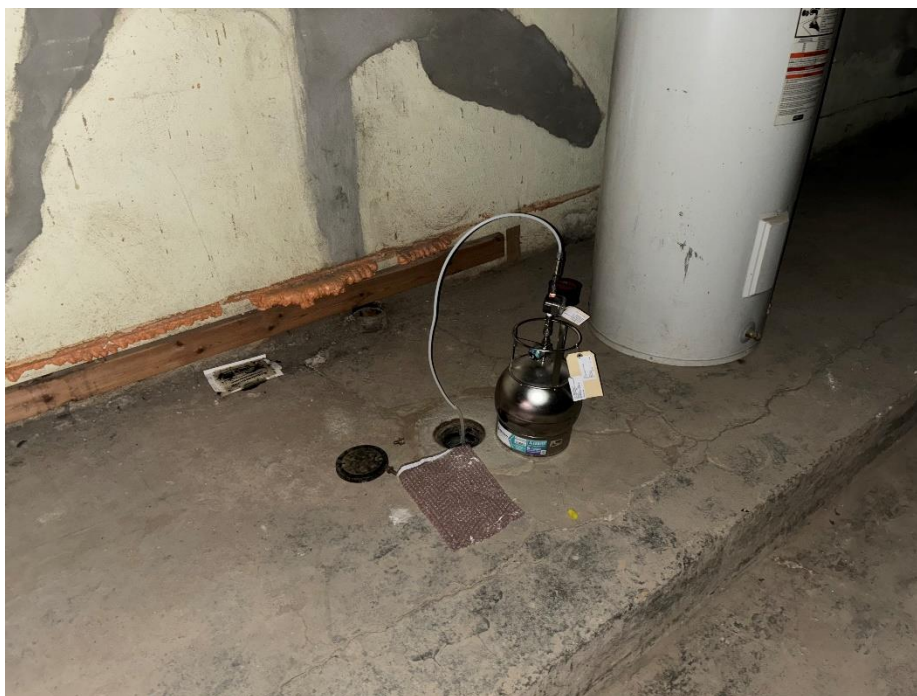
Photo 2, 12/12/2024: View of Langan collecting soil vapor sample MP02_121224 (facing southwest).
