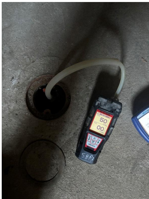
Photo 7, 12/12/2024: Langan collecting VOC readings from monitoring point MP-01 (facing down).
