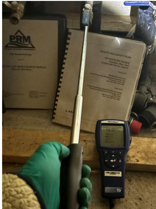
Photo 9, 12/12/2024: View of Langan collecting flow readings from the SVE manifold (facing north).
