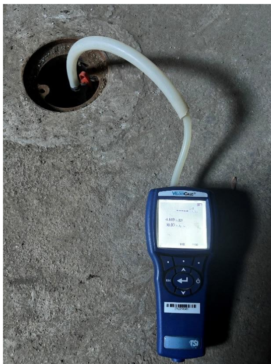
Photo 6, 12/12/2024: Langan collecting differential pressure readings from monitoring point MP-01 (facing down).
