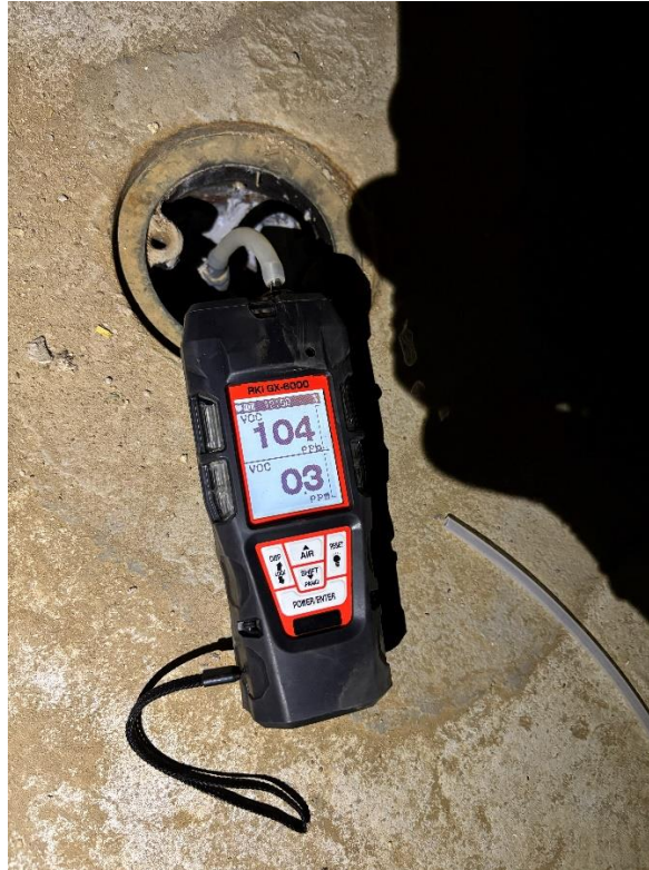
Photo 7, 12/12/2025: Langan collecting VOC readings from monitoring point MP-04 (facing down).
