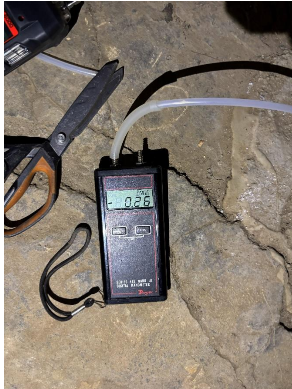
Photo 6, 12/12/2025: Langan collecting differential pressure readings from monitoring point MP-02 (facing down).
