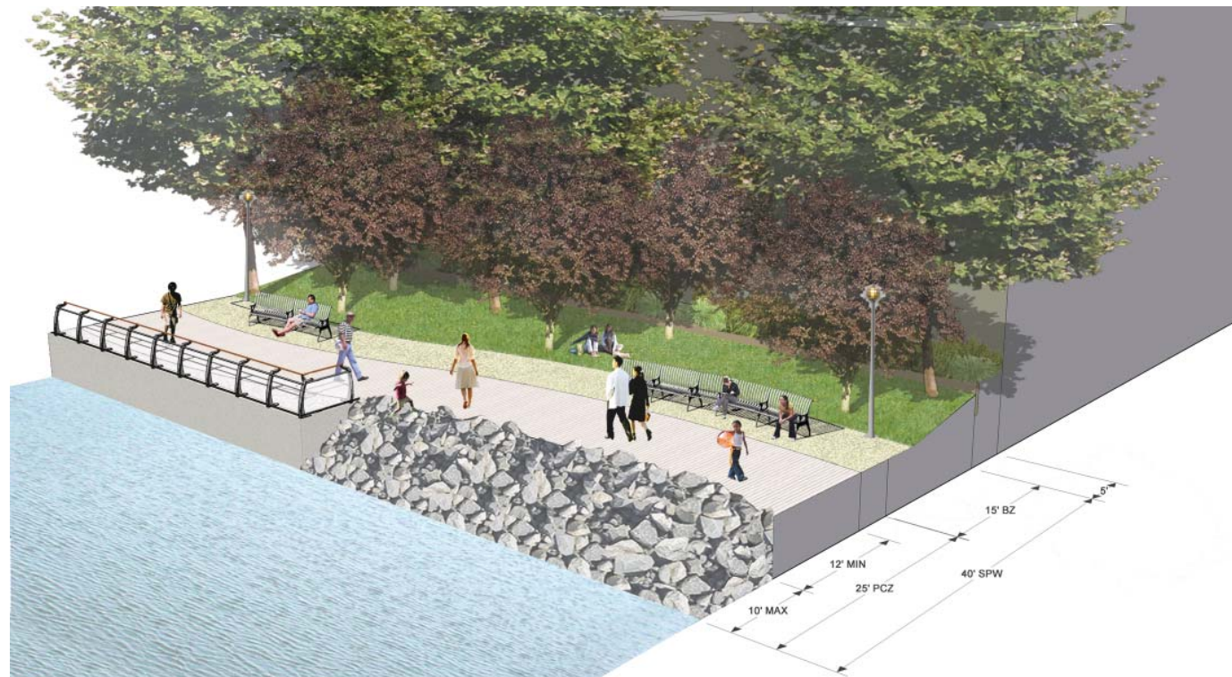
FIGURE 4-4: VIEW OF SHORE PUBLIC WALKWAY, WITH COMBINED RIP-RAP AND BULKHEAD WALL
