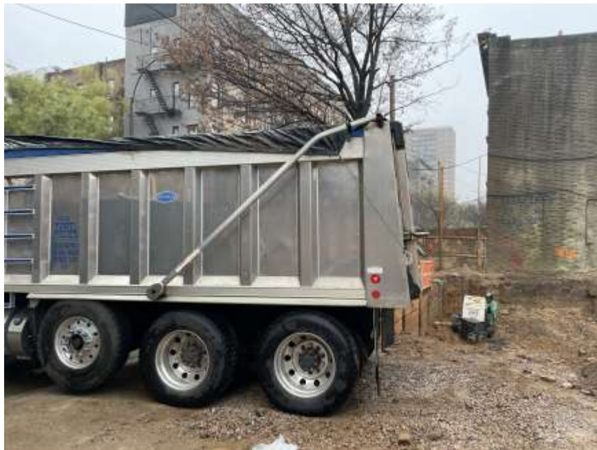
Photo 2: View of permitted tri-axle truck transporting non-hazardous fill for off-site disposal. Trucks were securely covered and tires washed prior to leaving the site (facing west).
