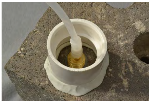
Figure 6. Water dam used for leak detection
