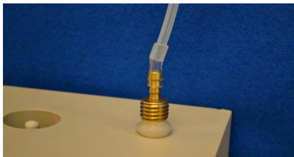
Figure 5. VAPOR PIN® sample connection
