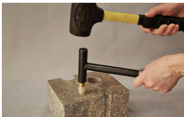
Figure 2. Installing the VAPOR PIN®
