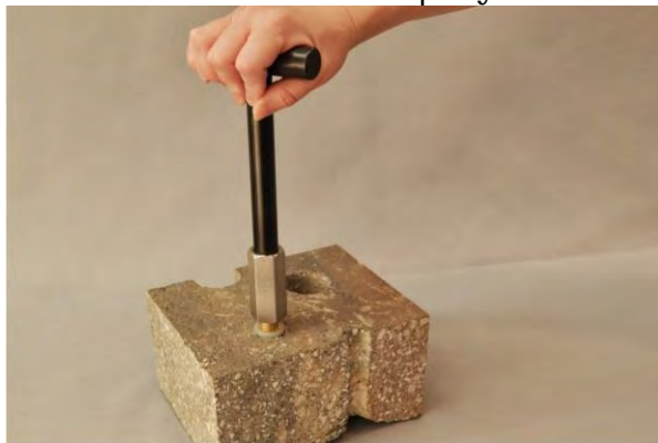
Figure 7. Removing the VAPOR PIN®
