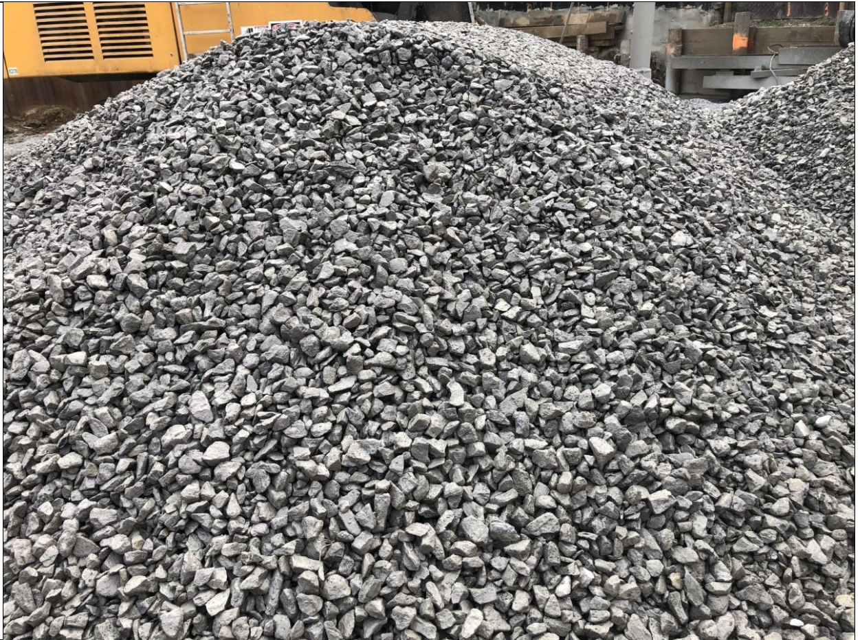
Photo 3 – Close-up view of the 0.75" stone imported from Lafarge-Ravena Quarry.
