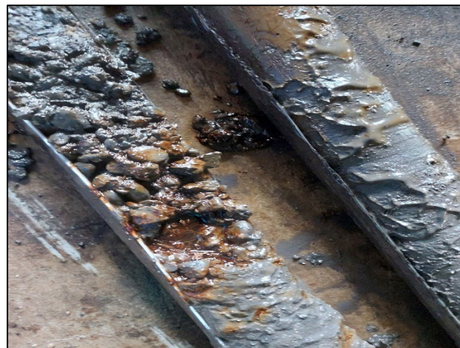
Photograph 8: Field evidence of petroleum contamination (NAPL globules) observed at soil boring RI-SB-09. (June 2022)
