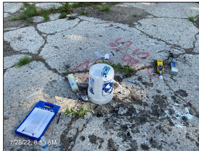
Photograph 18: Purging of a soil vapor point prior to the collection of soil vapor sample. (July 2022)
