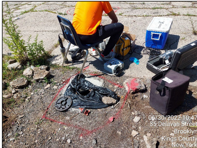
Photograph 13: Collection of groundwater samples at RI-MW-14 via low-flow sampling equipment. (June 2022)
