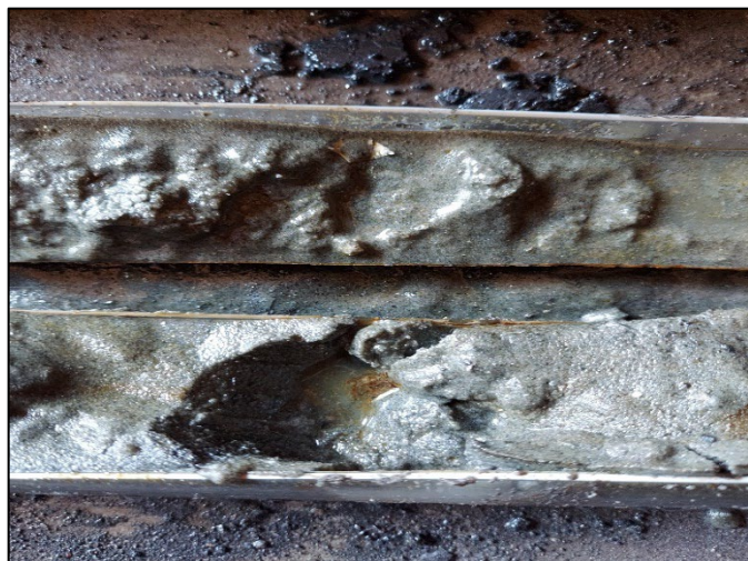
Photograph 7: Field evidence of petroleum contamination (NAPL globules) observed at soil boring RI-SB-11. (June 2022)
