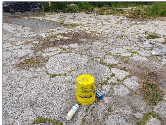
Photograph 10: Purging of a soil vapor point prior to the collection of soil vapor sample. (June 2022)
