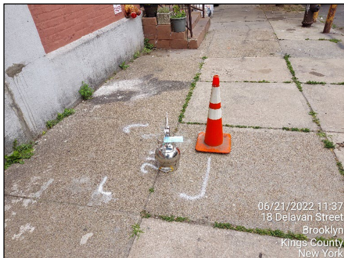
Photograph 11: Collection of an off-site soil vapor sample in the sidewalk along Delavan Street. (June 2022)
