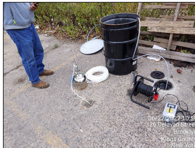
Photograph 12: Development of monitoring well RI-MW-17 and soil vapor sampling at RI-SV-17. (June 2022)
