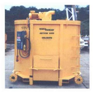
HIGHSHEAR<sup>™</sup> AGITATION TANKS ARE ELECTRIC DRIVE AND COME IN A VARIETY OF PADDLE SPEEDS AND TORQUES.
