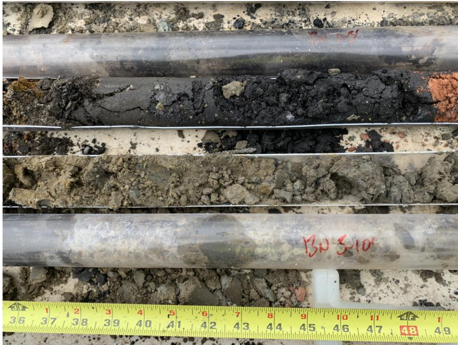
Photo 3, 5/07/2020: View of the macrocore samples recovered from soil boring LB13N.
