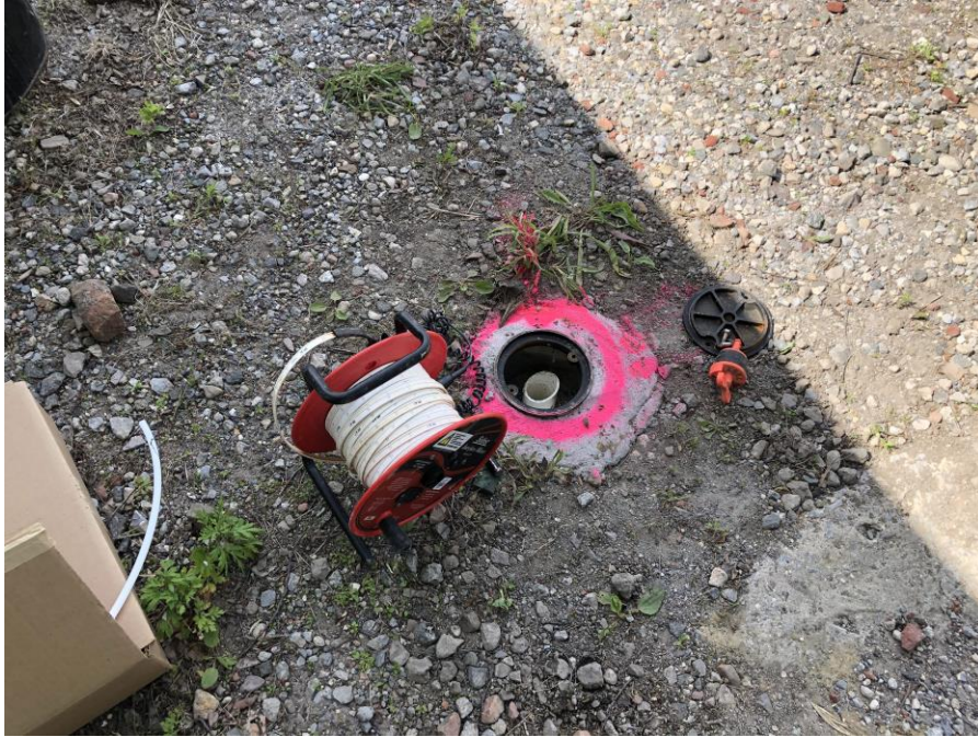
Photo 15, 5/20/2020: View of depth-to-water being gauged at monitoring well MW18 post-groundwater sampling.
