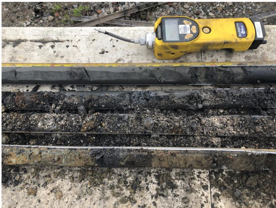
Photo 10, 5/11/2020: View of the macrocore samples recovered from soil boring LB25.
