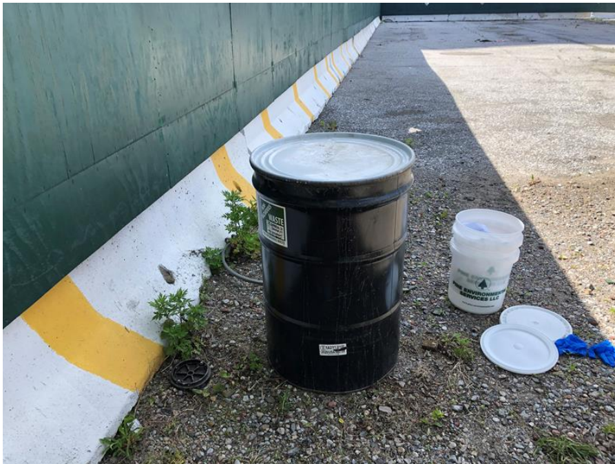
Photo 16, 5/20/2020: View of the properly labeled 55-gallon drum filled with purge water from groundwater sampling. The drum is staged on-site in preparation for off-site disposal (facing north).
