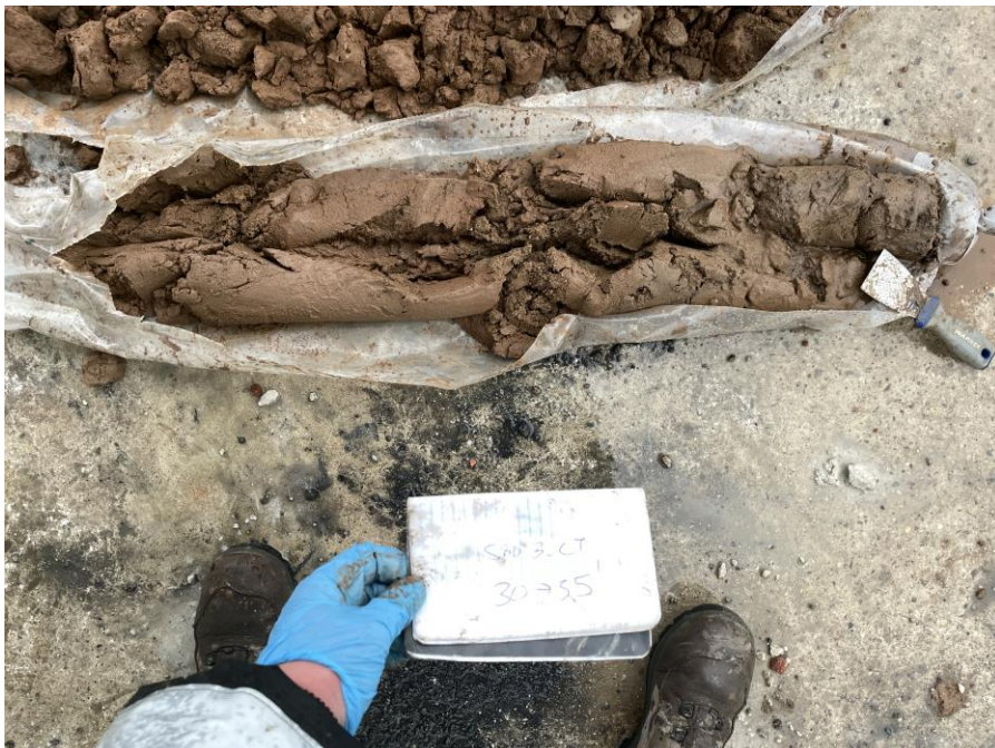
Photo 2: Soil screening at soil boring SB03_CT (facing down)
