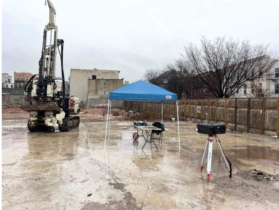
Photo 7: Perimeter air monitoring station set up downwind of SB03_CT on the 473 President Street site (facing east) 12/22/2022
