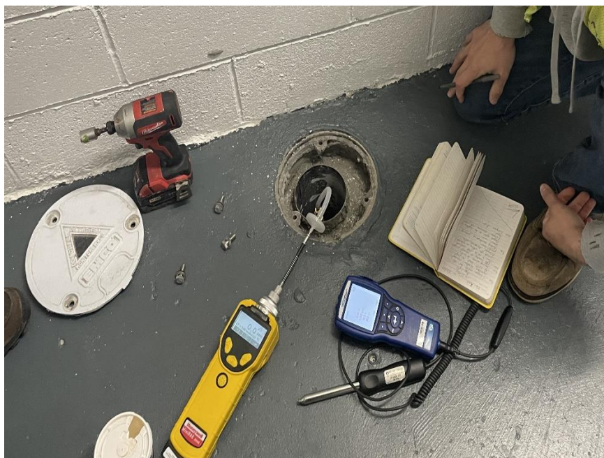
Photo 7: View of Langan collecting photoionization detector (PID) and vacuum readings at vacuum monitoring point MPA1.
