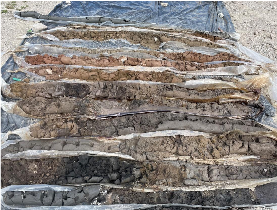
Photo 2: Recovery of soil at soil boring SB16 (facing down).
