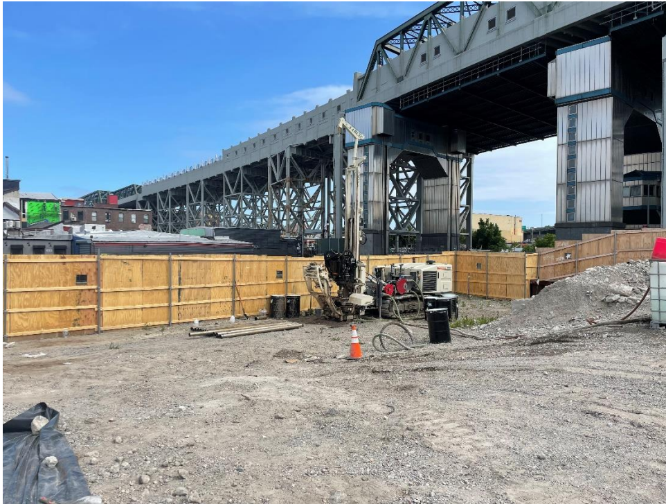
Photo 1: Geoprobe 8150LS® advancing soil boring location SB16 (facing southeast).
