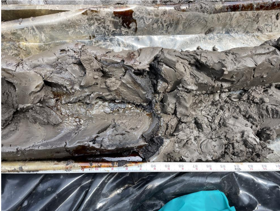
Photo 1: Coal tar impacts at boring location SB14 from about 57 feet bgs (facing down).
