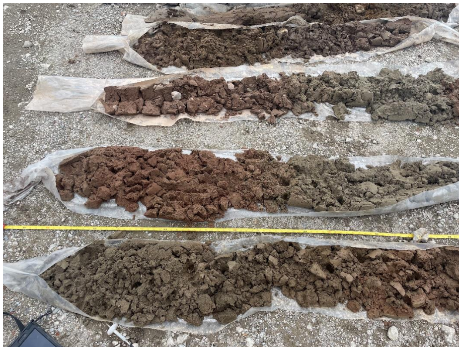
Photo 2: Recovery of soil at soil boring location SB17.
