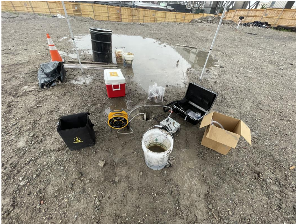
Photo 2: Groundwater sampling at location GW17 (facing south)
