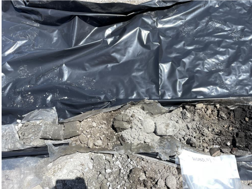
Photo 2: Recovery of soil at waste characterization borings (facing down).
