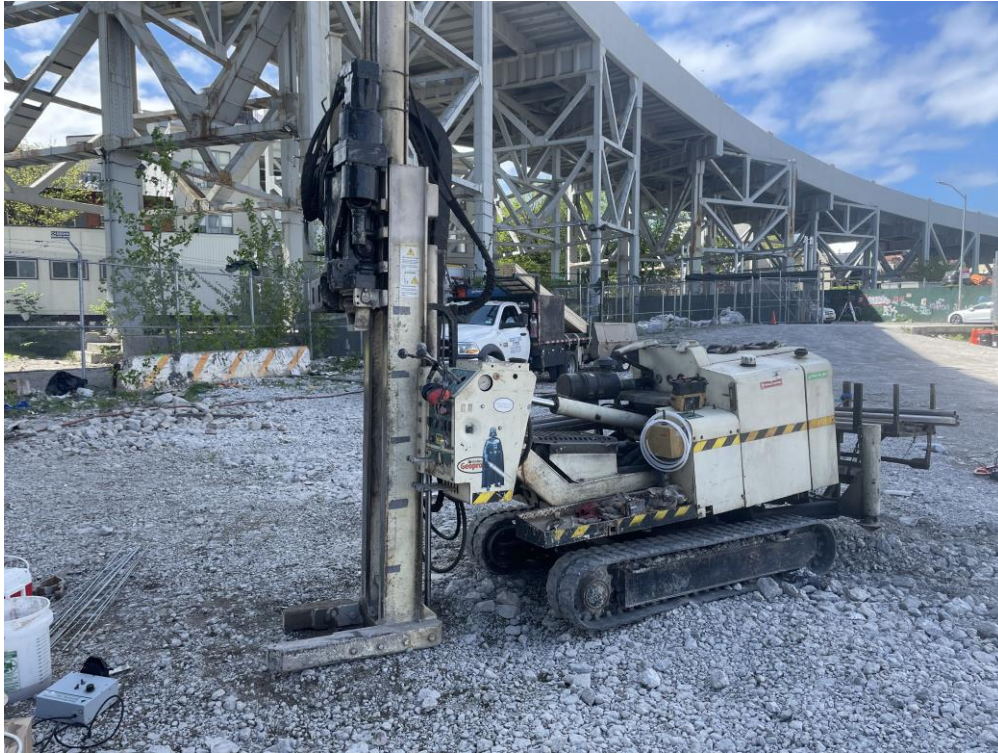
Photo 1: Geoprobe 6610DT® at GW18 location (facing northwest)
