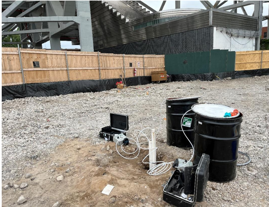
Photo 1: Groundwater sampling at SB21 (facing southwest)
