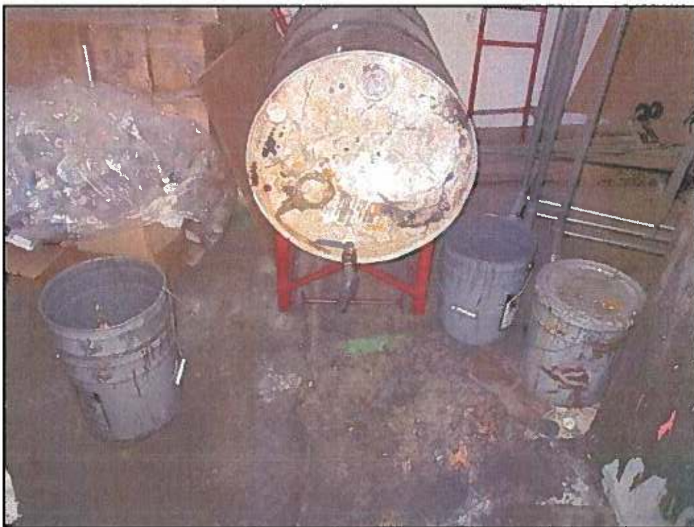
50 : View of a 55-gallon storage drum of methyl ethyl ketone, along with two 5-gallon buckets of paint and a bucket to catch drips from the drum (note de minimis staining on the concrete surface).
