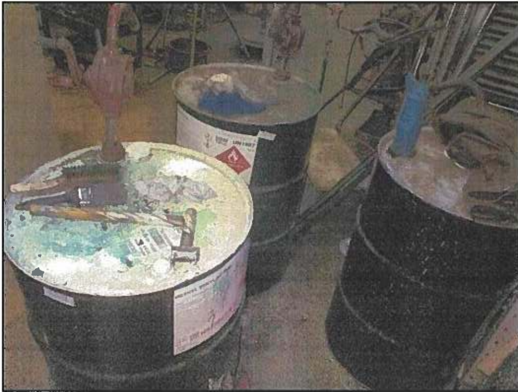
49 : View of three 55-gallon storage drums, two containing alcohol and one containing methyl ethyl ketone at 253 Bond Street.
