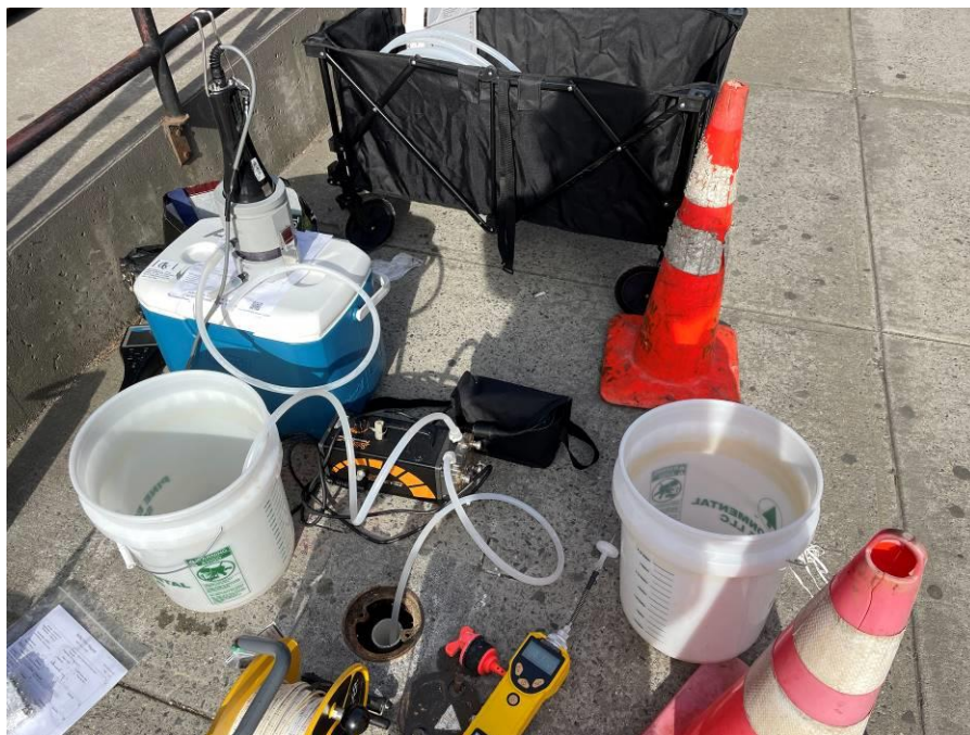
Photo 1: Groundwater sampling setup at monitoring well MW14S (facing northwest).
