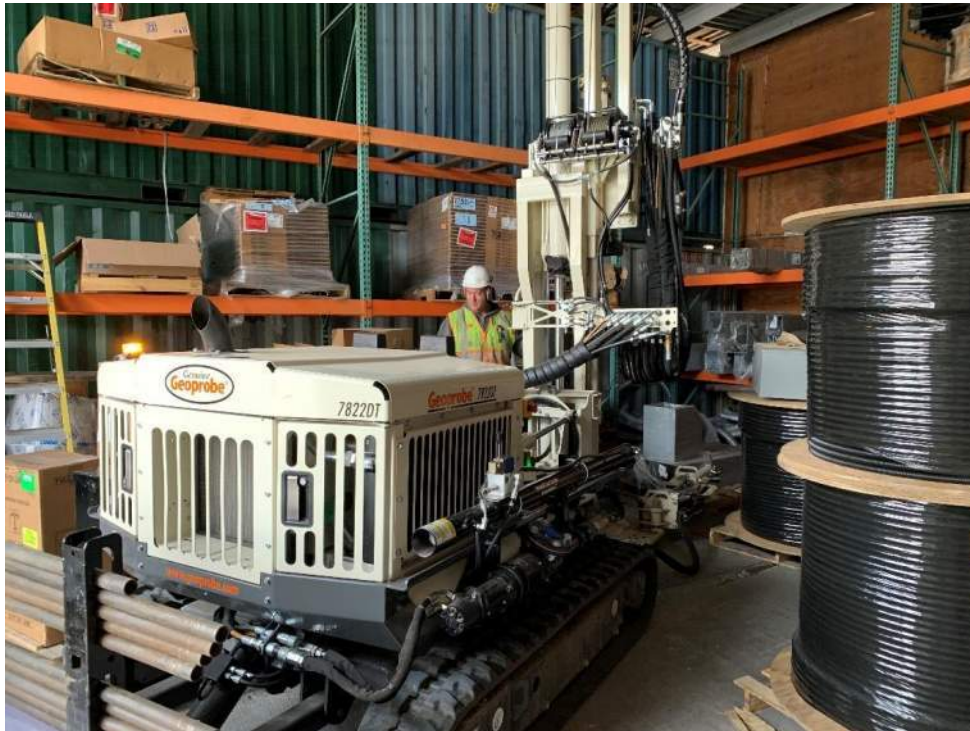
Photograph 1: View of Eastern drilling a soil boring with the Geoprobe® 7822DT track-mounted rig. Photo taken on January 28, 2020.
