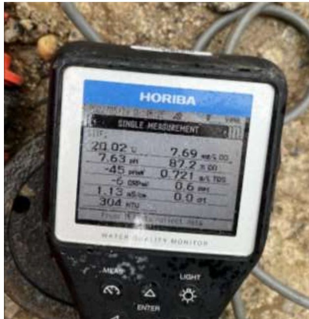
Photo 2: Water quality parameters measured on the Horiba U-52 at MW06 (facing south).
