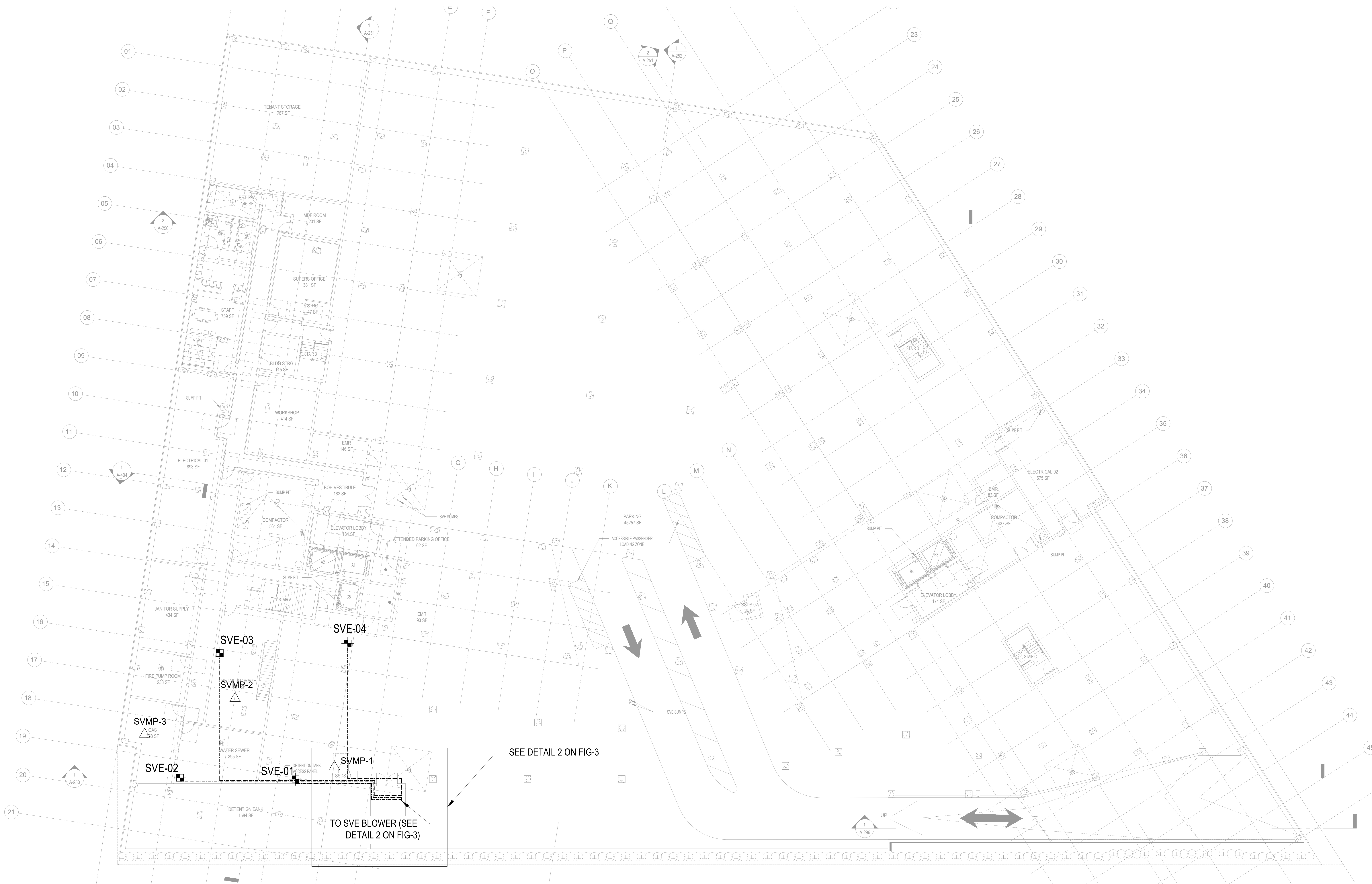
1 FIG-3 SOIL VAPOR EXTRACTION SYSTEM AS-BUILT LAYOUT SCALE IN FEET
